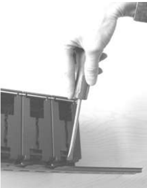
Figure 9 Removing the module from the DIN-rail
