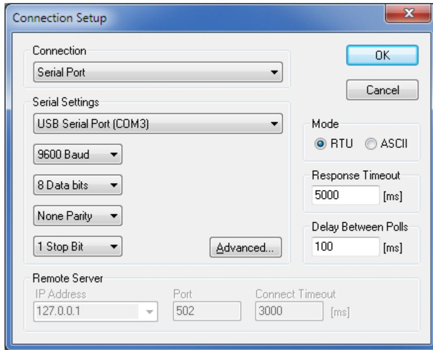
2.4.4 To read an input register, open or click on an Mbpoll window, and select Setup\Read\Write Definition from the menu bar. Set the Slave ID to match the Modbus Poll Address of the HMA. Set the Function to '04 Read Input Registers (3x)'. Using Appendices L through S, set the Address, Quantity and Display type in the pop-up dialog as required. Then click OK. The register value should appear in the Mbpoll window.
