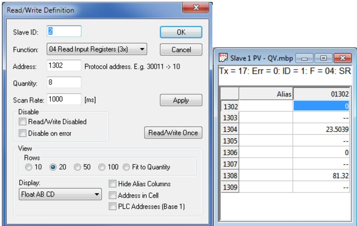
2.4.5 To read a holding register, open or click on an Mbpoll window, and select Setup\Read\Write Definition from the menu bar. Set the Slave ID to match the Modbus Poll Address of the HMA. Set the Function to '03 Read Holding Registers (4x)'. Using Appendices L through S, set the Address, Quantity and Display type in the pop-up dialog as required. Then click OK. The register value should appear in the Mbpoll window.
