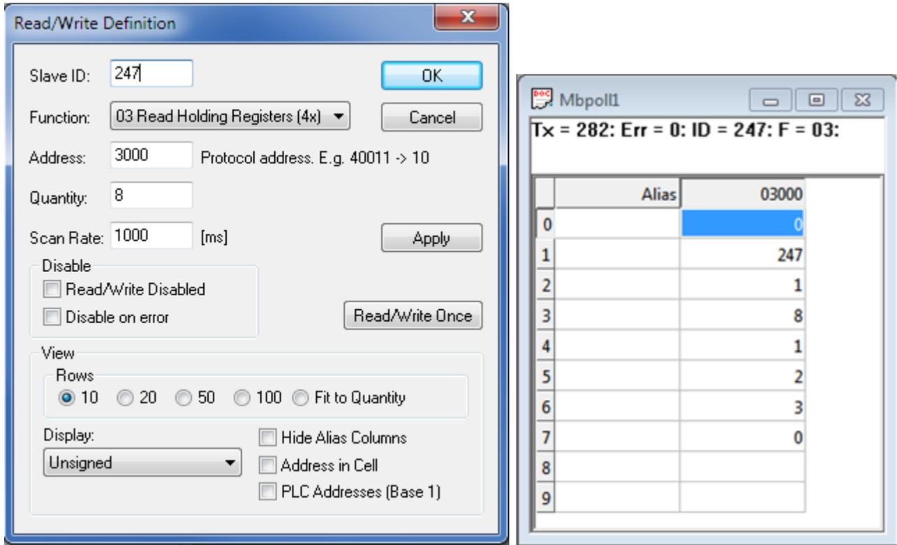
2.4.6 To write a holding register, double-click on the register value displayed in step 2.4.6. Enter the new value and click on 'Send'. Confirm that the new value appears in the Mbpoll window.
