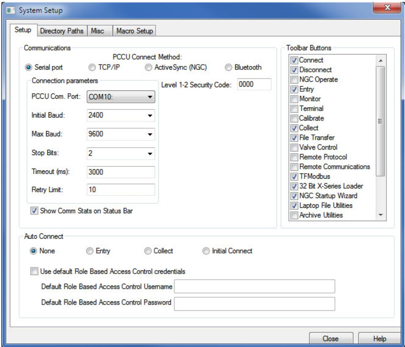
16.3.3 Select the COM port number corresponding to the XRC. The proper COM port number can be identified by navigating to the Device Manager in Windows and expanding the Ports entry.
