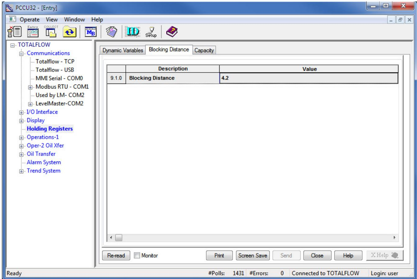
16.5.8 Note the Register number displayed in the first column of the table. It will be used when setting the Request Block in a later step.
