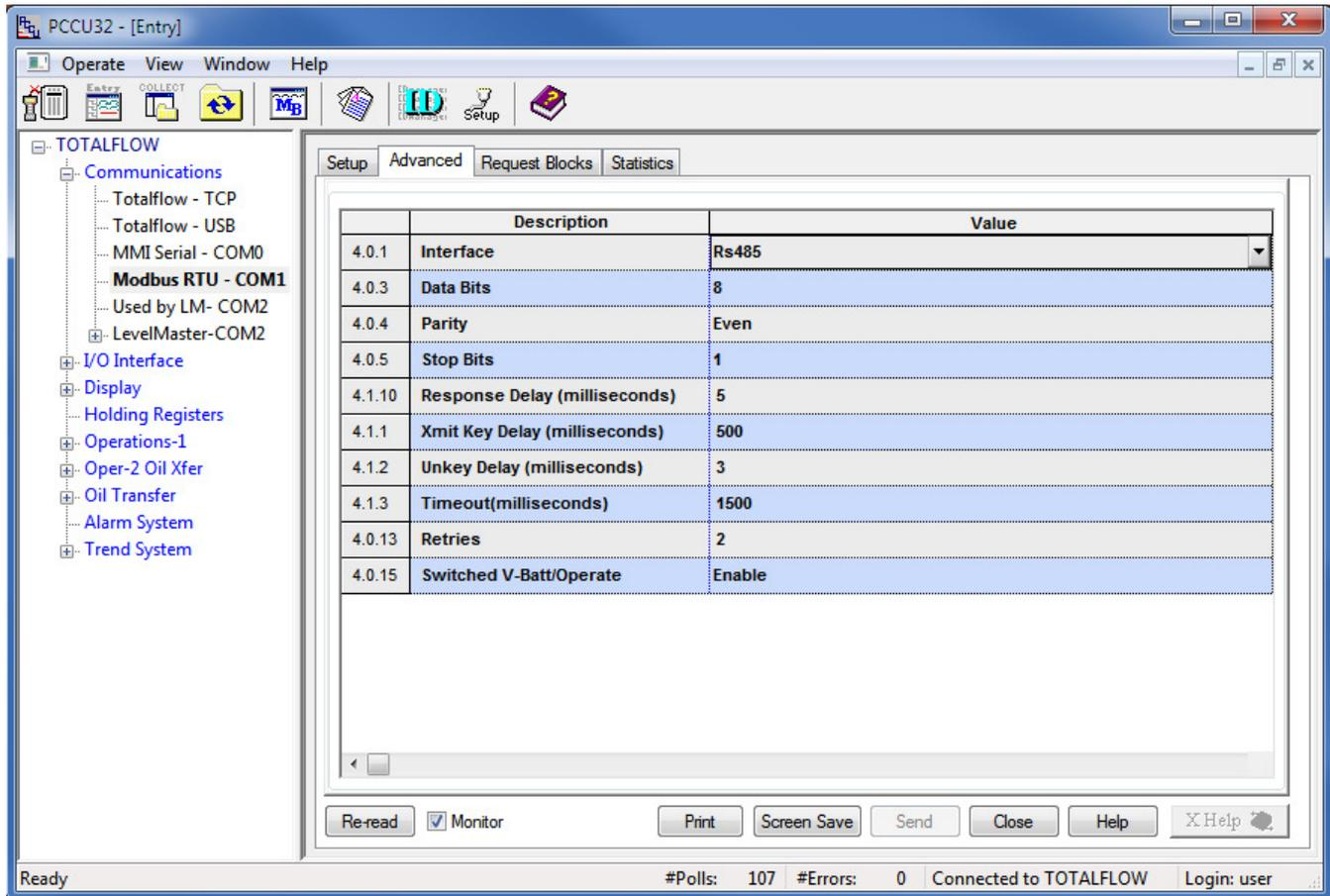
16.4.14 Ensure that the Unkey Delay is less than 7 milliseconds as the HMA typically responds within about 8 milliseconds. If the Unkey Delay time is too long, the XRC will start listening for a response after the HMA has already started transmitting. As a result, the XRC will not recognize the response.
