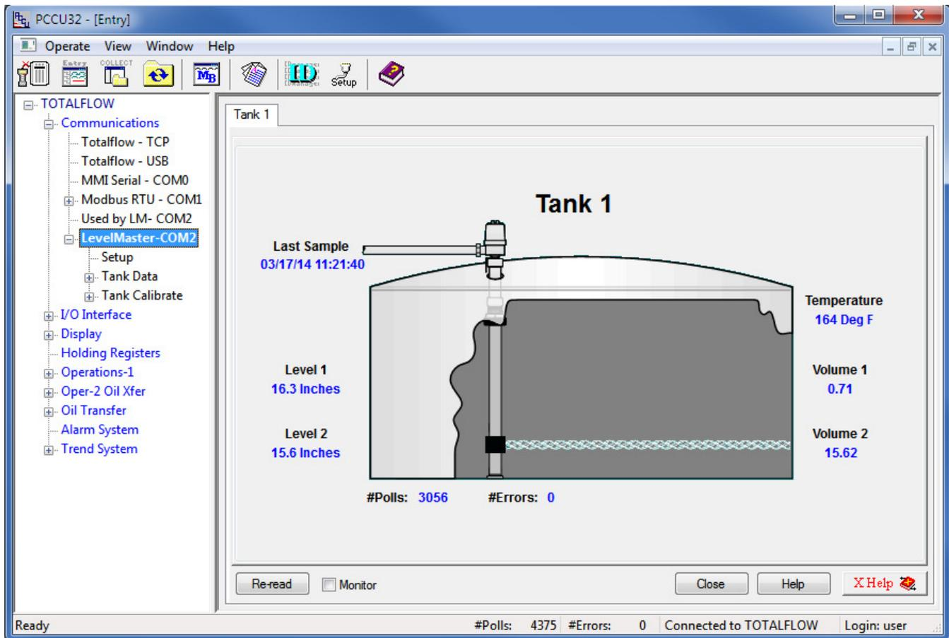
17.4.21 Click on Re-read to obtain a single set of readings from the HMA, or check the Monitor checkbox to repeatedly read values from the HMA at the Interval specified in the Request Blocks tabs in step 18.4.9.
