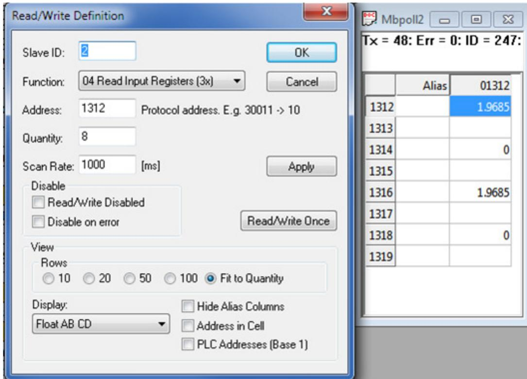
8.4.17 Ensure that the values displayed match the values shown on the selected transmitter's local user interface.
