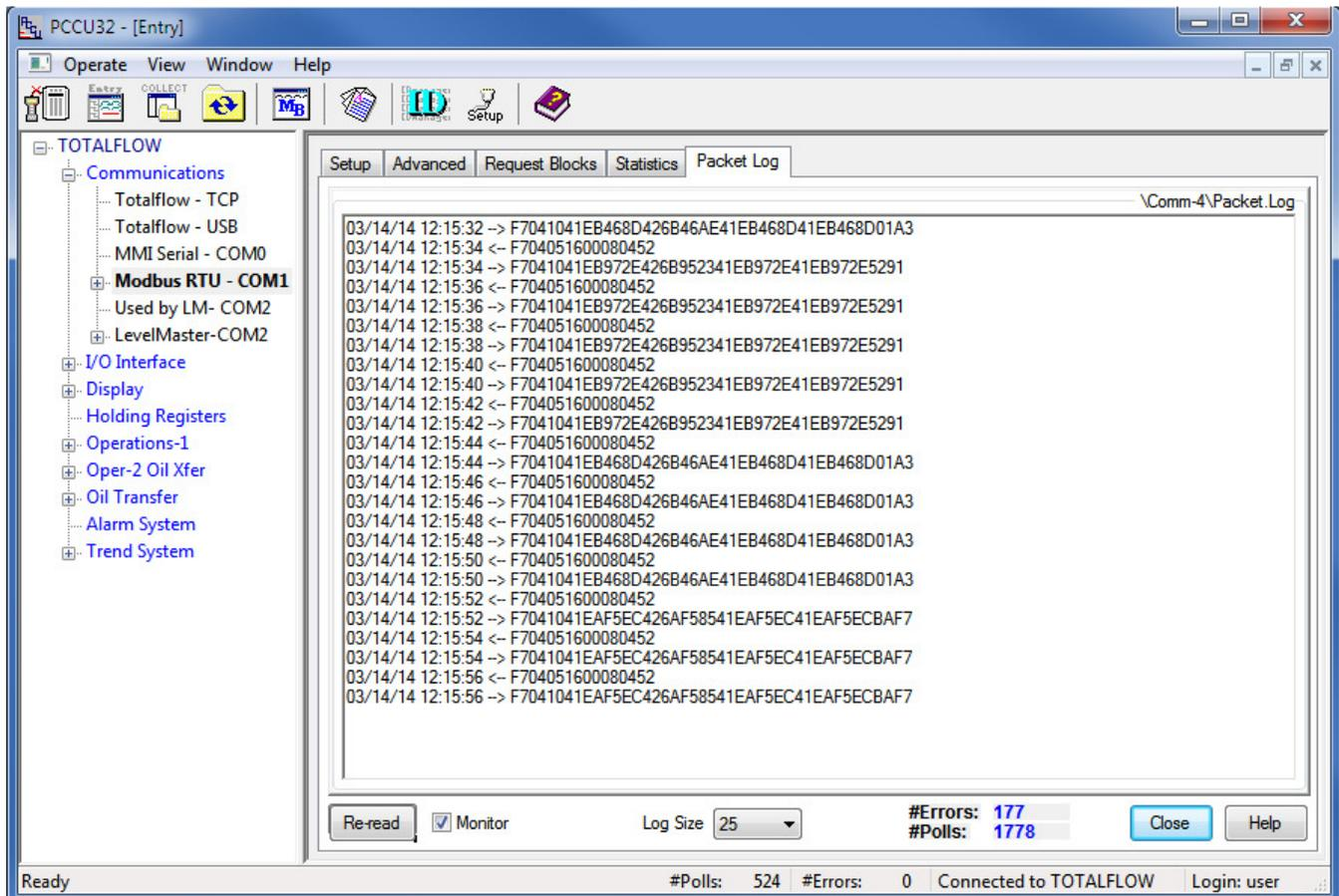
16.4.25 Set the Log Size to 25, and check the Monitor checkbox. The log should start updating with the XRC commands being sent out and the responses from the HMA.
