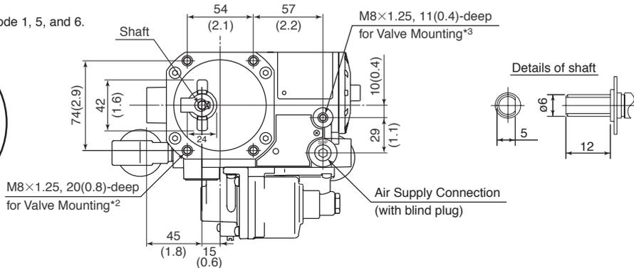
\*2: Attached with 4 mounting bolts (M8, 25 mm) and spring washers (applicable 3 to 6 mm thick brackets).
