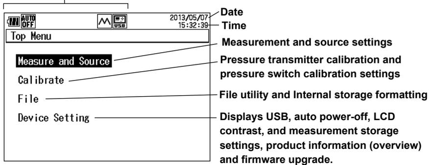
Selecting **Measure and Source** from the top menu shows a pressure, voltage, and current measurement and voltage and current source displays. The top half of the display shows the pressure measurement display (Display1), and the bottom half displays the current and voltage measurement/source display (Display2).
