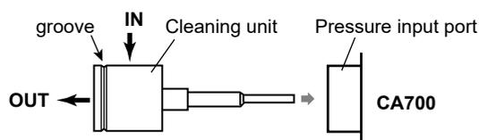
1. Connect a cleaning unit to the CA700 pressure input port by tightening the connection by hand.
