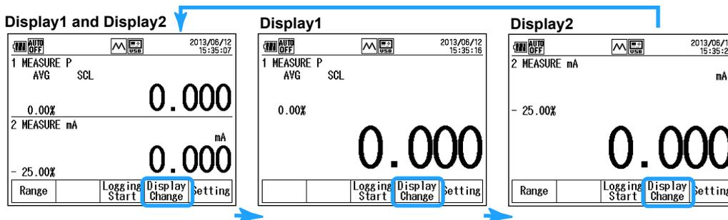
When only Display1 or Display2 is showing, pressing Setting (F5) will show the corresponding setup display.
