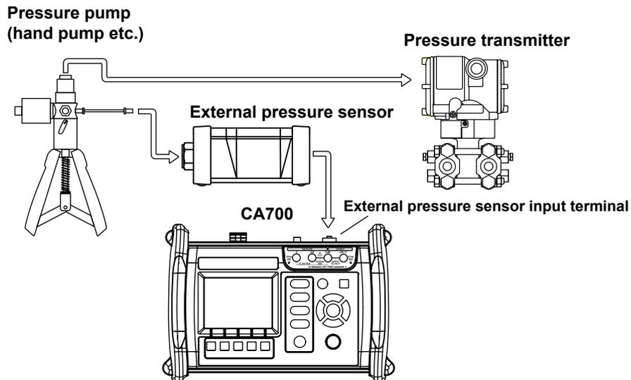
Power on the CA700. When the external pressure sensor is recognized successfully, the icon indicating that sensor appears on the screen of the CA700.
