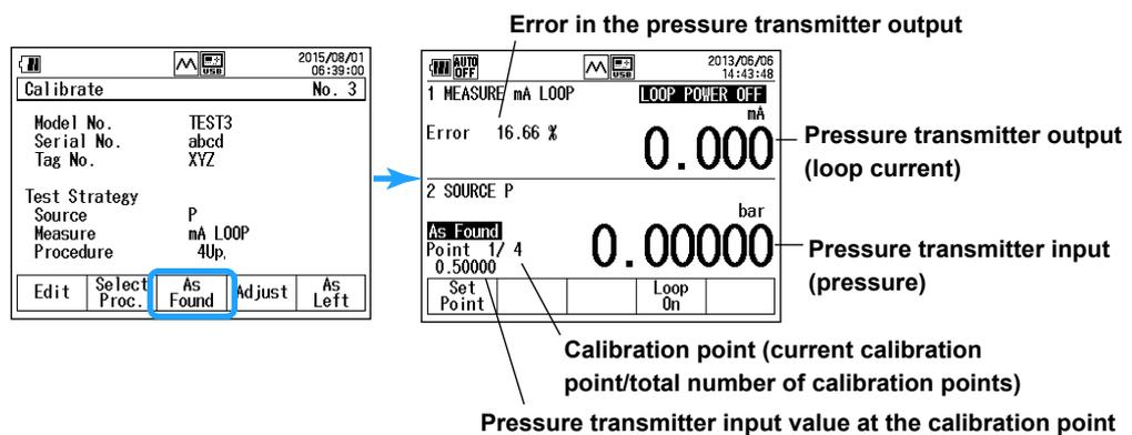
4. Press **Loop On (F4)**. The CA700 outputs a 24 VDC loop voltage and measures the loop current.
