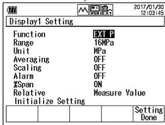
**Leak pressure measurement display when the external pressure sensor is used**
