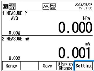
**Loop current (mA LOOP) measurement display**
