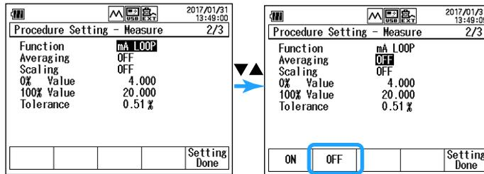
10. Turn scaling off. To use scaling, select **ON**, and press **ENTER**. A scaling setting menu appears.
