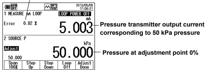
16. Press **Span100% (0%) (F1)**, **Step Up (F2)**, and **Step Down (F3)** to change the adjustment point, and repeat steps 13 to 15.
