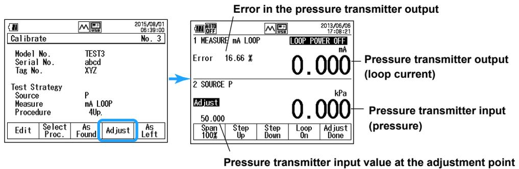
12. Press **Span100% (0%) (F1)**, **Step Up (F2)**, and **Step Down (F3)** to set the adjustment point.
