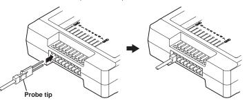
Removing the Probe Tip Remove the earth leads (for main unit) in the same manner.
