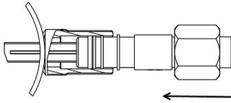
6. Tighten the nut to the specified torque.
