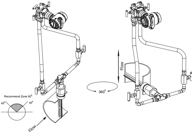
**Figure 6. Flowmeter Orientation for Steam**
