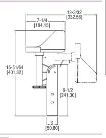
The SERIES MARK II Wind Speed Indicator indicates wind speed directly on the liquid filled scale reading in both miles per hour (0-80) and Beaufort scale (1-12). A metric model is also available, which reads the same as above, but reading 0-130 kilometers per hour. The Mark II Wind Speed Indicator is an accurate, economically priced option for measuring wind speed.
