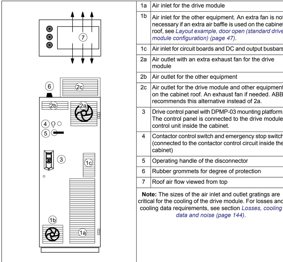
■ Layout example, door open (standard drive module configuration)
