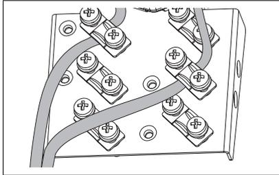
11. Connect the conductors to the appropriate detachable terminals of the control unit. See the default I/O diagram in chapter [Control unit \(page 107\)](#). Use shrink tubing or insulating tape to contain any stray strands. Tighten the screws to secure the connection.
