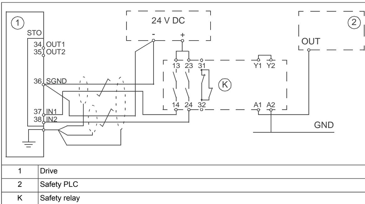
Multiple ACQ580-04 drives, internal power supply
