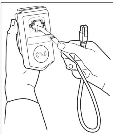
**Note:** When a PC is connected to the control panel, the control panel keypad is disabled. In this case, the control panel acts as a USB-RS485 adapter.
