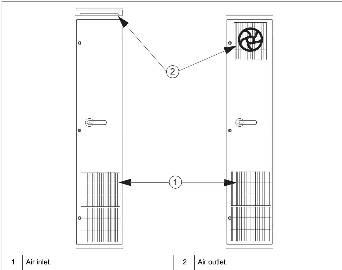
Arrange the cooling air flow through the components according to the technical data. See the specifications for:
