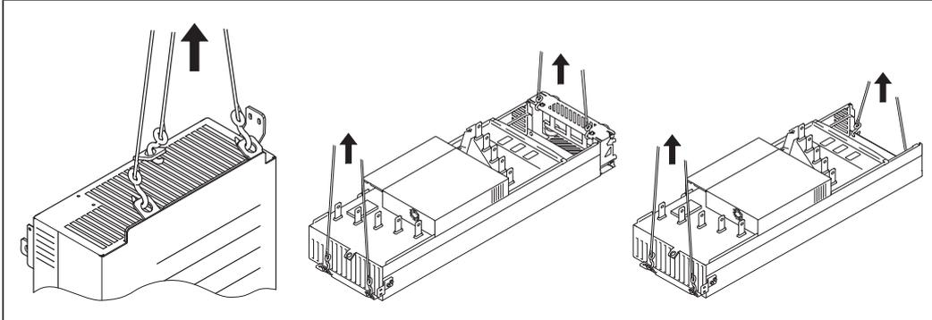
Make sure that the module does not topple over when you move it on the floor: Open the support legs by pressing each leg a little down (1, 2) and turning it aside. Whenever possible attach the module also with chains. Do not tilt the module. It is heavy and its center of gravity is high. The module overturns from a sideways tilt of 5 degrees. Do not leave the module unattended on a sloping floor.
