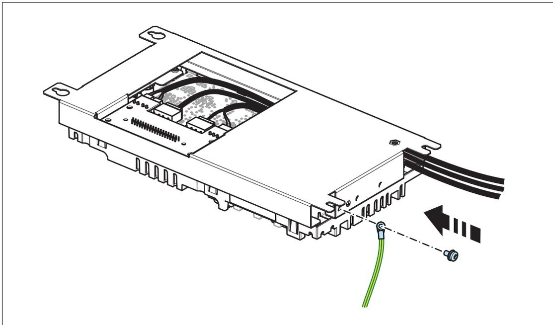
6. The kit includes a plate for the customer cable screens. Attach the small bracket (a) first, then the full clamp plate (b).
