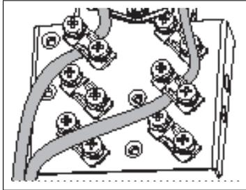
7. Connect the conductors to the appropriate detachable terminals of the control unit. See chapter [Control unit \(page 107\)](#) for the default I/O connections of the drive module. Use shrink tubing or insulating tape to contain any stray strands. Tighten the screws to secure the connection.
