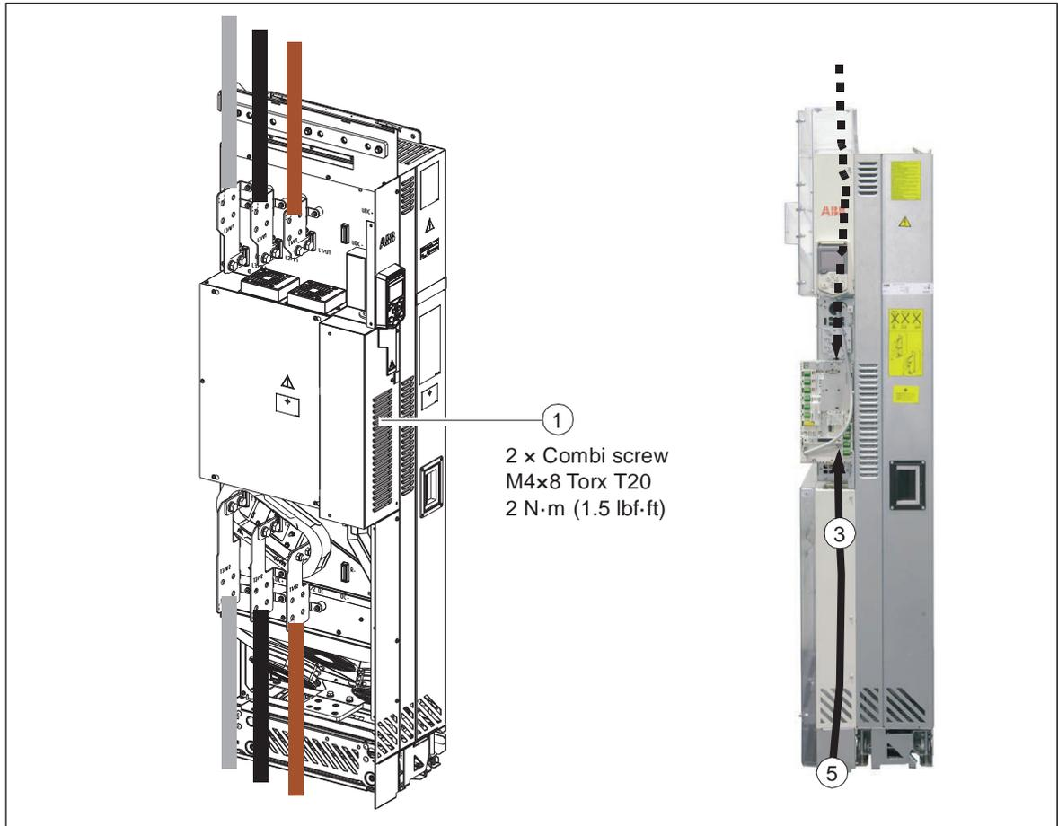
1. Remove the middle front cover of the drive module.
