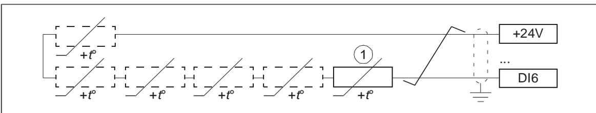
1 One to six PTC thermistors connected in series
