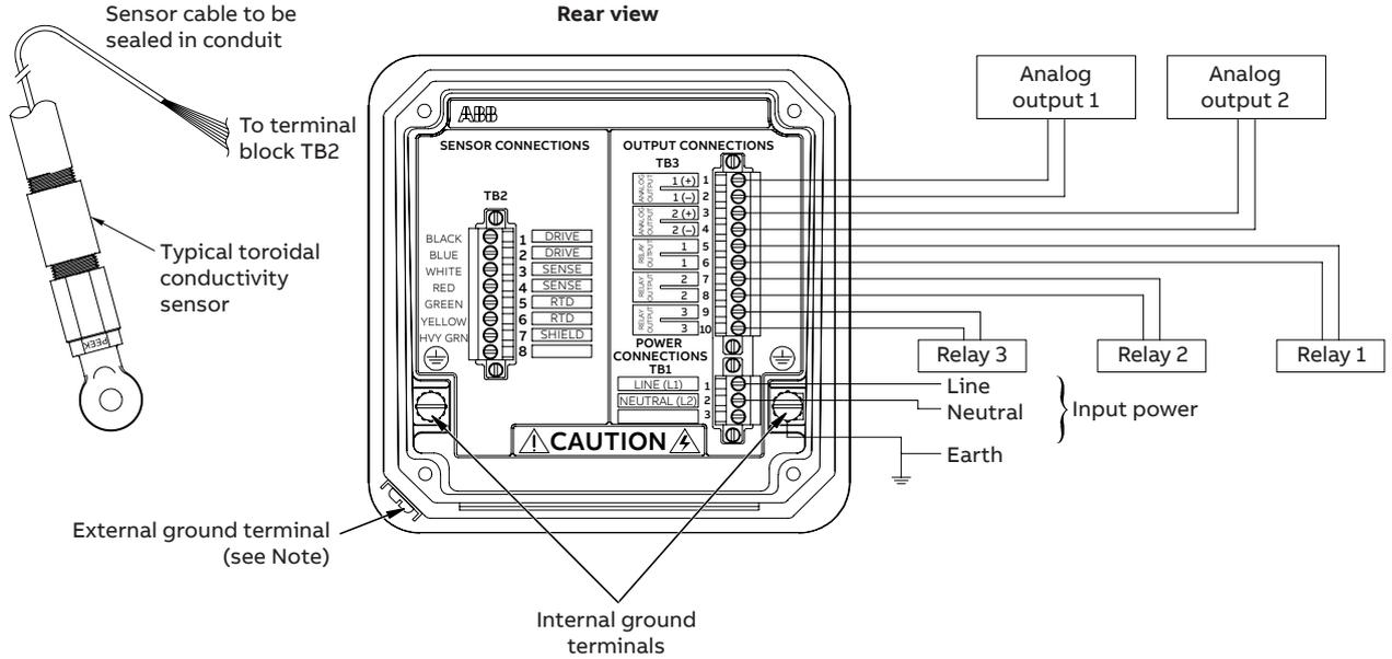
**Note.** To avoid interference, connect the transmitter enclosure to earth (ground) using a large area conductor (ground strap) ensuring resistance is less than 0.2 Ω.
