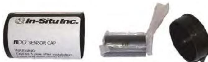
3. Align the arrow on the cap with the index mark on the probe and firmly press the cap onto the probe, without twisting, until it seals.
