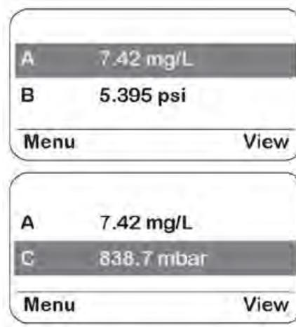
Lines labeled A and B refer to probes A and B. C refers to measurements made by the analyzer. See also [Section 4.2](#).
