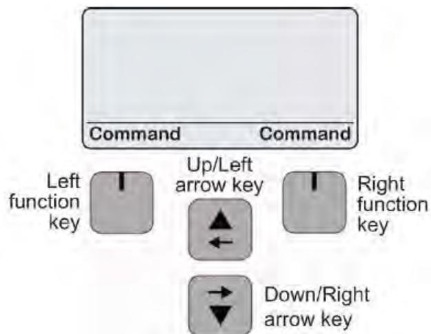
The **Up/Left** arrow key has three functions: it moves the cursor to the left; it moves the cursor up a list; it increases the value of a digit. The **Down/Right** arrow key has three functions: it moves the cursor to the right; it moves the cursor down a list; it reduces the value of a digit. The left and right function keys perform the operation shown in the screen immediately above the key.
