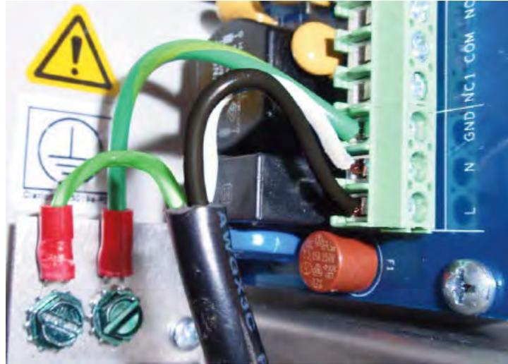
5. Connect the live and neutral power wires to the *L* and *N* terminals.
