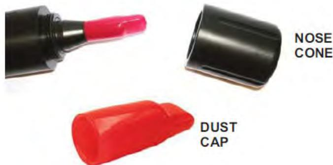
2. Remove the RDO sensing cap from its shipping/storage sleeve.
