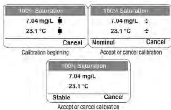
Note the *Calibration Beginning* icon next to the mg/L reading. As the reading stabilizes, the bar in the icon shrinks. When the word *Nominal* appears, the stabilization is almost complete, and the calibration can be selected at this point by selecting *Nominal*. However, for best results, wait until *Stable* appears.
