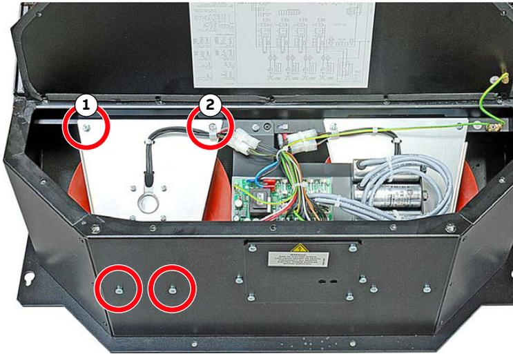
3. Remove the fan from the housing and unscrew the fan from the mounting bracket.
