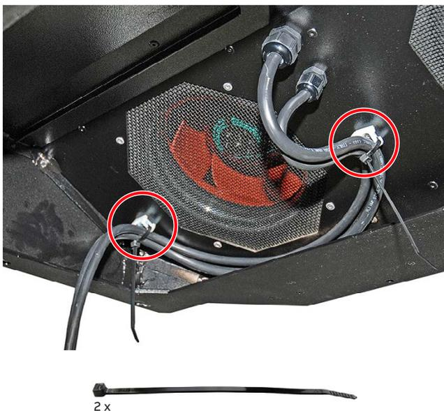
3. Loop a length of the cables and fasten them to the cable tie mount (circle).
