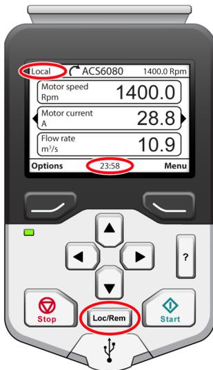
2. Press the STOP key (⏹) on the control panel to stop the motor.
