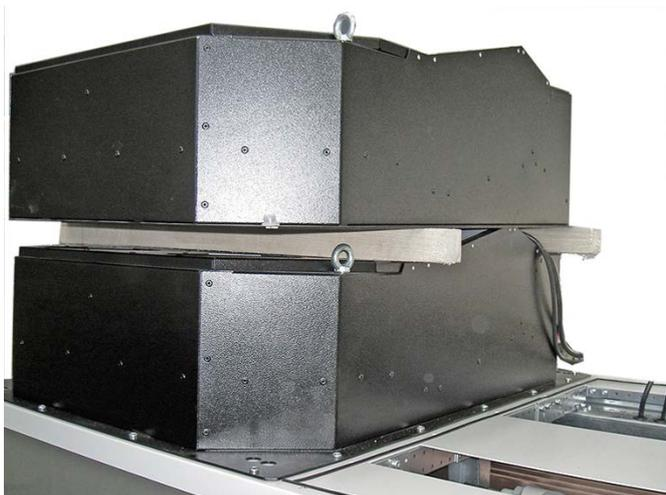
6. Join the DC busbars with the supplied installation material.
