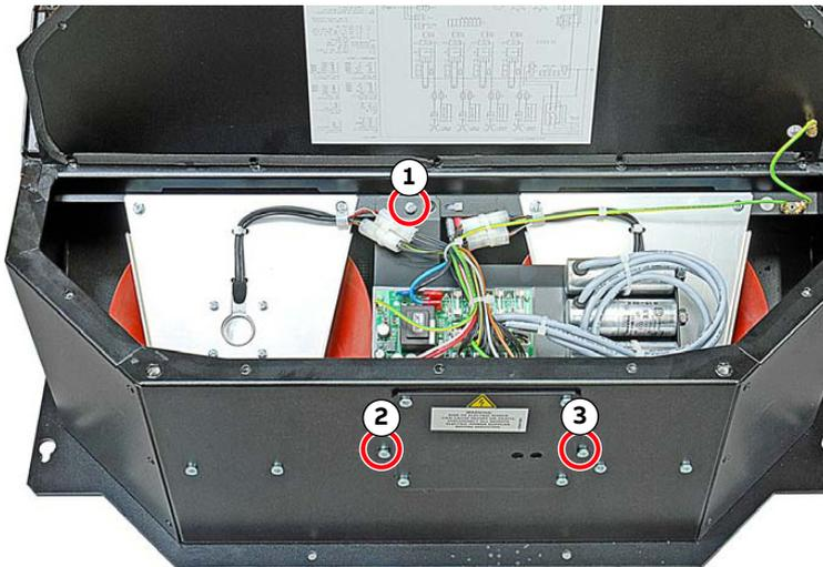
4. Take out the circuit board mounting bracket and place it on the heat exchanger housing.
