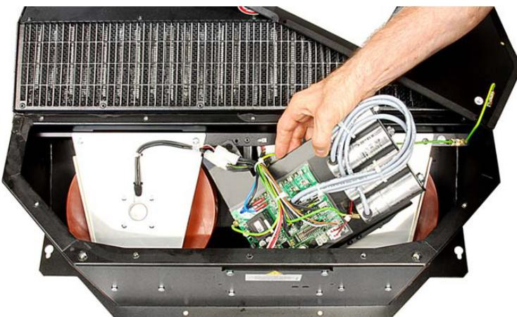
5. Disconnect the ground wire (1), cut off the cable tie (2), unplug the plug-in connectors (arrows), and unscrew the screws (3, 4, 5 and 6) fixing the fan mounting bracket to the housing.
