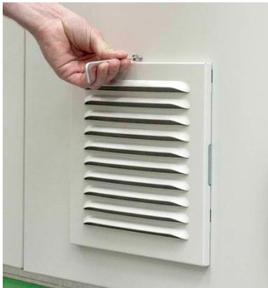
3. Slide the cover up and pull it out of the slots.
