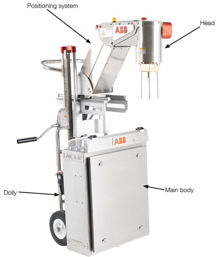
Figure 9: The LiMCA III analyzer
