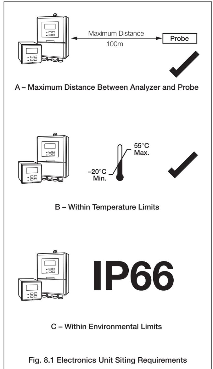
8.2 Mounting the Electronics Unit
