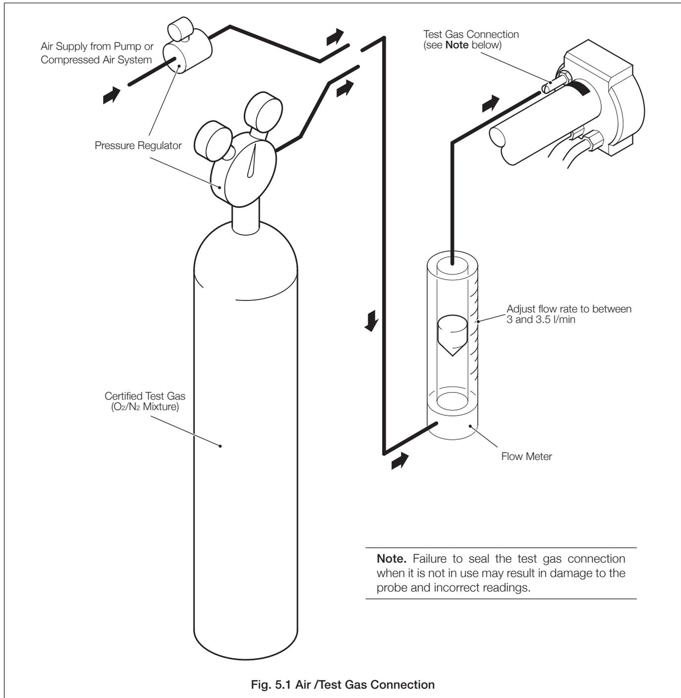
**Note.** Before commencing a gas calibration procedure, the electronics unit and probe must be switched on and allowed to operate for at least one hour to allow the system to stabilize thermally.
