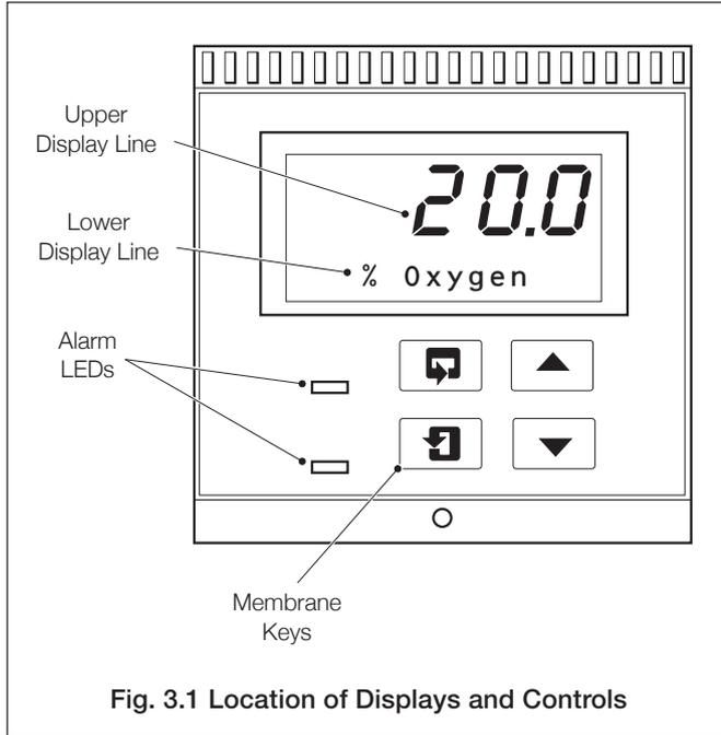
Fig. 3.1 Location of Displays and Controls
