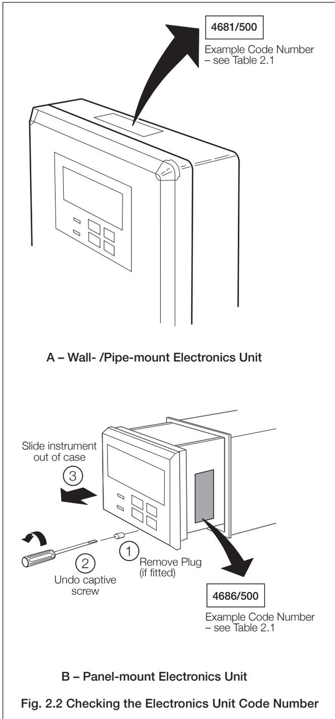
Fig. 2.2 Checking the Electronics Unit Code Number
