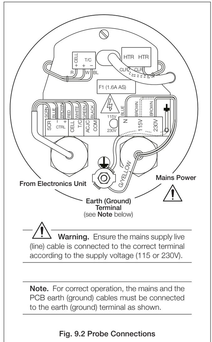
**Note.** The cable glands supplied with the probe may be replaced by any 1/2in. NPT cable entry gland that is certified to  $80^{\circ}\text{C}$  and classed as watertight.
