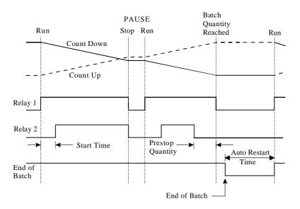
The Batch Controller can also be programmed, during Calibration, to either count up from zero on each batch, or to count down from the preset batch quantity.
