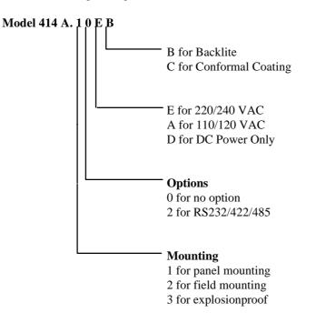
The Model Number of the instrument is displayed on first entering the Calibration Mode (see Section 5).
