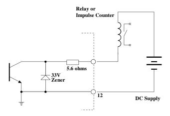
Driving an External Relay or Impulse Counter
