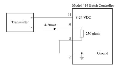
Transmitter Powered by the Flow Computer
