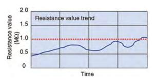
With this functionality, even inexperienced engineers can determine when adhesion occurs. Periodic maintenance is not necessary, as maintenance is only needed when impedance reaches the threshold level.
