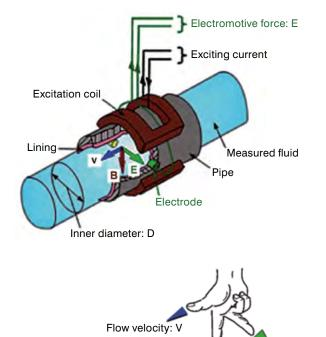
Magnetic field (magnetic flux density): B
