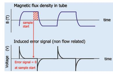
very beginning of the Yokogawa magmeter development that a commercially acceptable solution was needed that would combine the advantages of both methods to produce a new excitation concept:
