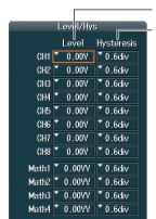
Set the level used to detect the state of each signal.
