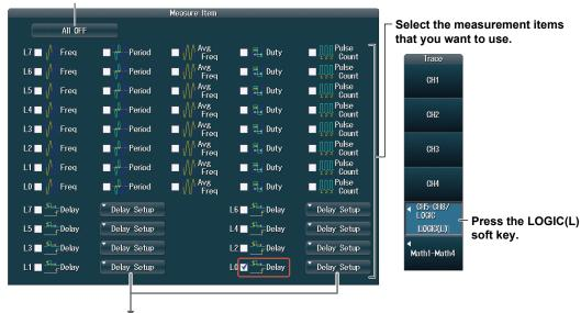
Configure the measurement of delay between waveforms.
