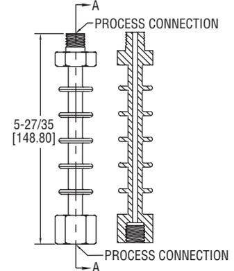
The **SERIES A-240/A-250** Perforated and Spiral Cooling Towers protect pressure instruments during high temperature applications. Both the spiral and perforated styles are made with 316L SS, and are available with various process connections in NPT or BSPP style. Both Cooling Towers are ideal for use with pressure gages, switches, and transmitters where the process media temperature exceeds the rating of the instrument.
