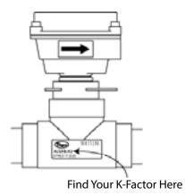
If the EFS2 Series meter is ordered with a saddle or weldolet fitting, find your K-factor in the chart below.
