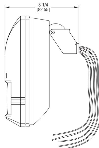
The Model OSW-100 Wall Mount Occupancy Sensor is an infrared sensor designed to automatically control a HVAC ventilation system. A unique dual delay processor eliminates false triggers due to short-term occupancies. The Model OSW-100 has a wide 110° viewing angle to capture movement up to 49.2 ft (15 m) away.
