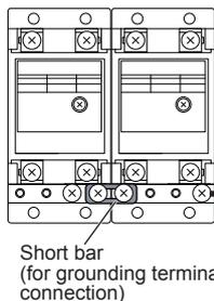
Grounding for serial installation of arresters is to connect grounding terminals of neighboring arresters to each other and touch ground at one point from last arrester according.
