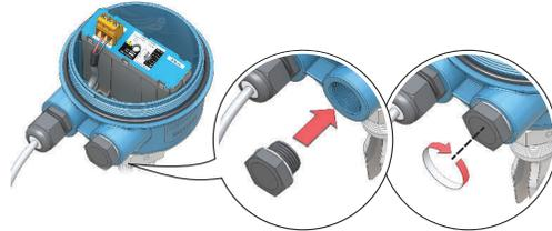
9. Attach and tighten the cover.
