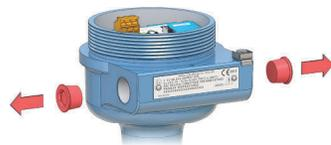
4. Pull cables through the cable gland/conduits.
