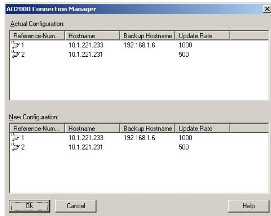
Click on "File → Connection Manager" to open the above window which makes it possible to manage all connections at a glance. Using the drag&drop function you can move connections from the "Actual Configuration" to the "New Configuration" to edit them comfortably there.
