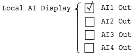
Because the Model 705 transmitter has four Analog Input blocks any or all of which may be used in particular applications, a Transducer block parameter controls which AI block Out values will be displayed.
