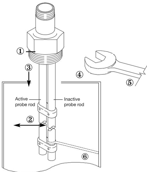
**NOTE:** If the transmitter is to be installed at a later time, do not remove the protective cap from the probe. Do not use sealing compound or TFE tape on probe connection to transmitter as this connection is sealed by a Viton® O-ring.
