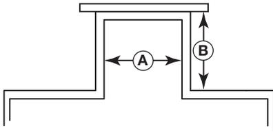
2. Ratio of Diameter: Length (A:B) is 1:1 or greater; any ratio <1:1 (e.g., a 2" x 6" nozzle = 1:3) may require a Blocking Distance and/or DIELECTRIC adjustment (see Eclipse Installation & Operating Manual 57-600, Section 2.6.5.2, Measurement Type: Level and Volume).
