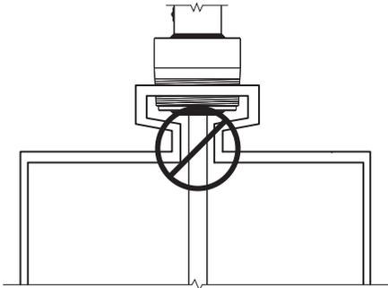
**3.4.3.1 To install a Model 7xF rigid single rod probe:**
