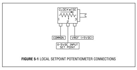
It is recommended that a potentiometer between 5K to 10K ohm and capable of at least 10-turns or more for adjustment be used. Use the control potentiometer to command the percentage of flow desired.
