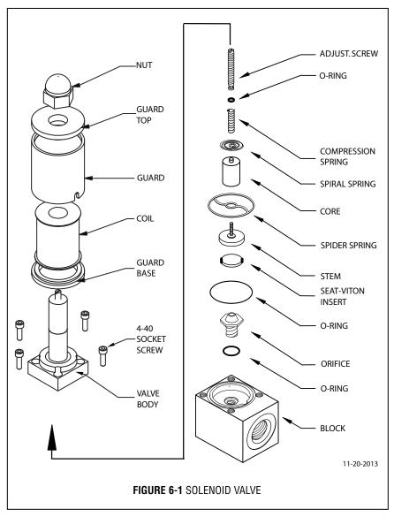
Various corrosive gases may demand more frequent replacement of VITON® O-rings and seals inside the valve. Be sure to use an elastomer material, appropriate for your specific gas application. Contact your distributor or Dwyer for optional sealing materials available.
