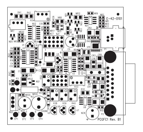
GFC-1100-09, 2100-09 /1111, 1131, 1133 /2111, 2131, 2133, 1142 /2142 CONTROLLER PC BOARD (TOP SIDE)
