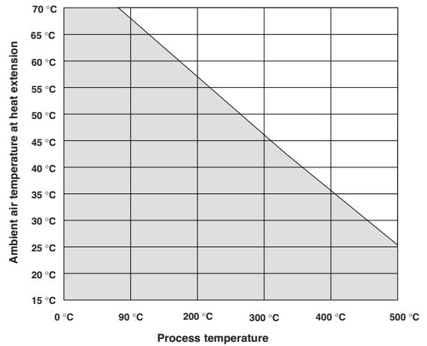
The heat dissipation graph depicts the maximum temperatures at which the extension, P/N 89-6593-001 can be used effectively.
