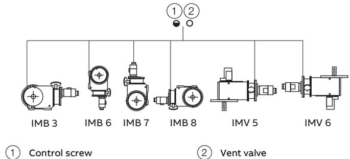
Figure 3: Permissible mounting positions
