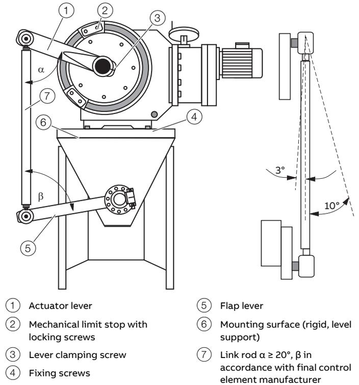
Figure 4: Component lever actuator
