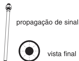
SONDA COAXIAL GWR
