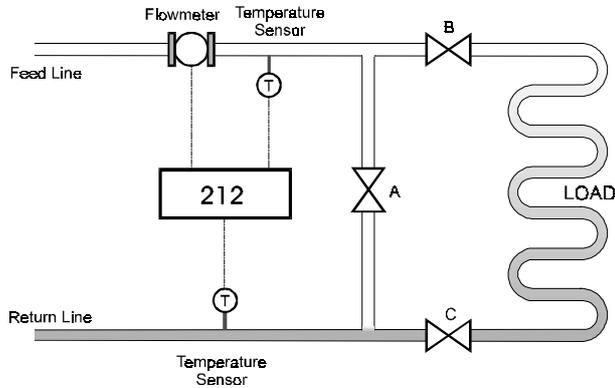
To compensate for any offset in the temperature sensors the Model 212 must be put into the Set-up Program mode. The bypass valve "A" is then opened and the valves "B" and "C" are closed.
