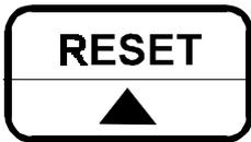
If the Reset function is enabled during set-up, the RESET key, when held for 5 seconds, will reset all totals and the operating time.
