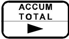
Displays the accumulated (non-resettable) totals for Energy, Volume, operating time (elapsed time) and Energy total for log entries.
