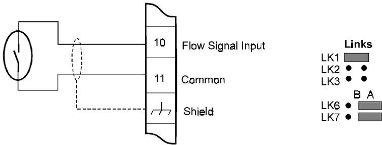
3. Coils eg. mV signals from turbine flowmeters or paddlewheels.
