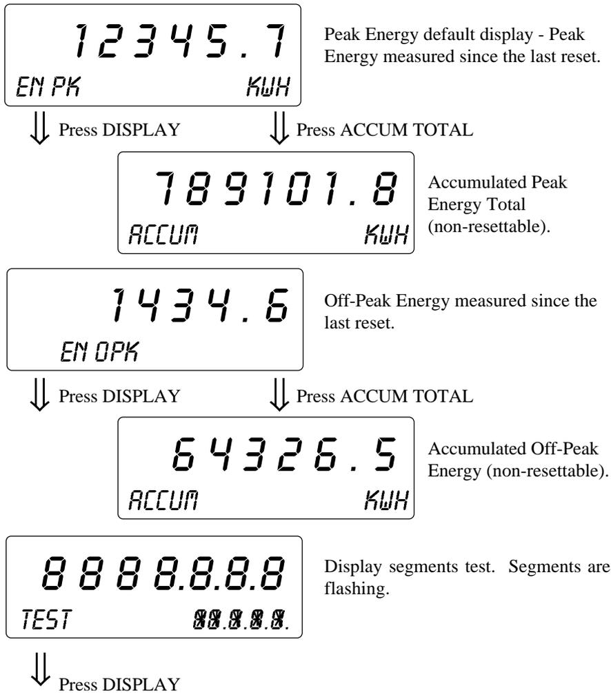
For continuation of displays refer to Section 3.1.1 Normal Operation.
