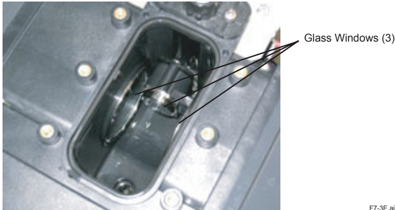
Figure 7.3 Inside the Detector Measurement Cell
