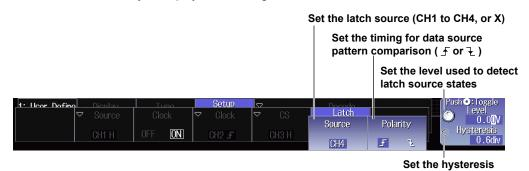
Specify the timing at which the data source pattern sampled in sync with the clock source is compared with the specified pattern.
