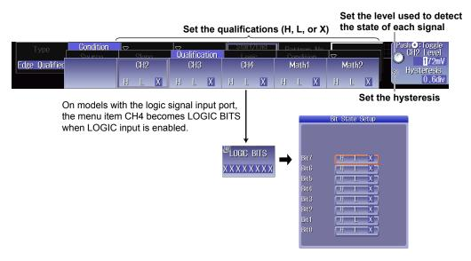
Setting the Hysteresis and the Level Used to Detect the Signal State for Each Signal (Level/ Hys)
