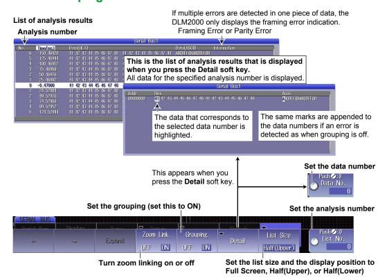
Data before the trigger position (on the left side of the waveform display) is assigned analysis numbers in descending order (-1, -2,and so on). Data after the trigger position (on the right side of the waveform display) is assigned analysis numbers in ascending order (0, 1, 2,and so on).
