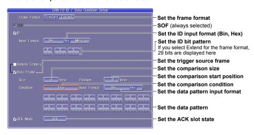
When the Comparison Condition Is Data = a; Data ≠ a; a ≤ Data; Data ≤ b; a ≤ Data ≤ b; or Data < a, b < Data</li>
