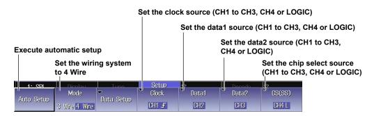
The auto setup feature automatically configures the level and hysteresis and then triggers on the SPI signal's first data byte.
