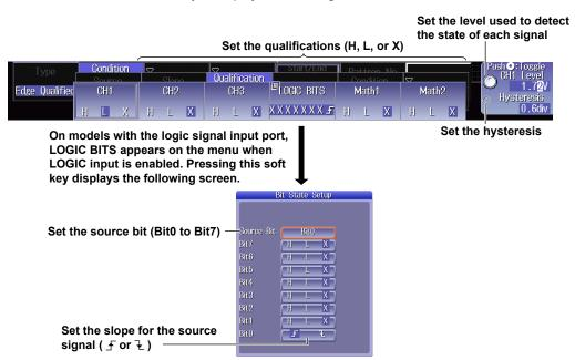
Setting the Hysteresis and the Level Used to Detect the Signal State for Each Signal (Level/Hys)
