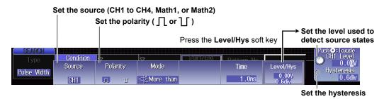
. When the Source Is LOGIC (On models with the logic signal input port)
