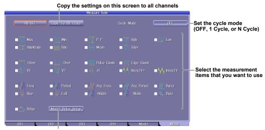
Configure the measurement of delay between waveforms
