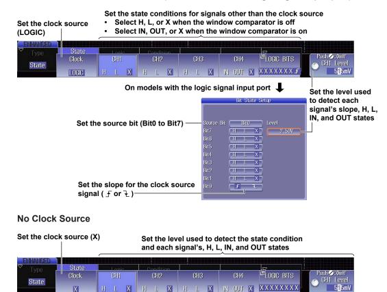
The same menu appears as that shown on the previous page for when the clock source is set to a channel from CH1 to CH4. Because there is no clock source, you can specify all of the signal states from CH1 to CH4 and LOGIC as state conditions.
