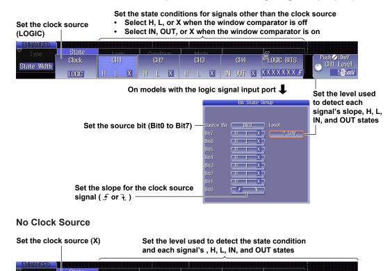
The same menu appears as that shown on the previous page for when the clock source is set to a channel from CH1 to CH4. Because there is no clock source, you can specify all of the signal states from CH1 to CH4 and LOGIC as state conditions.
