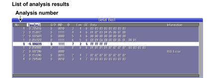
Data before the trigger position (on the left side of the waveform display) is assigned analysis numbers in descending order (–1, –2, and so on). Data after the trigger position (on the right side of the waveform display) is assigned analysis numbers in ascending order (0, 1, 2, and so on).
