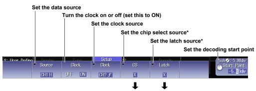
\* The chip select source and latch source can only be set on 4-channel models.
