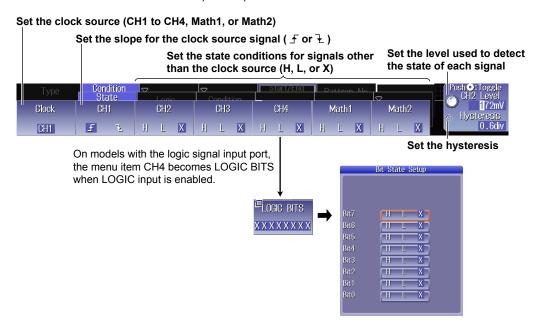
When the Source Is LOGIC (On models with the logic signal input port)
