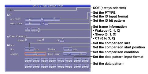
When the Comparison Condition Is Data = a; Data ≠ a; a ≤ Data; Data ≤ b; a ≤ Data ≤ b; or Data < a, b < Data</li>
