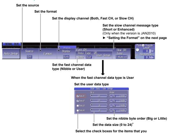
\* The total number of bits for Data1 to Data4 is up to 24. If you try to exceed the total number of bits, the data size of other pieces of Data is reduced.
