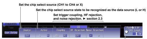
Set the level used to detect chip select source states
