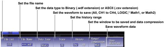
\* The DLM2000 saves data from the CH4 or LOGIC waveform, depending on which channel's key is illuminated.
