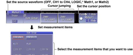
You cannot select CH4 while the LOGIC key is illuminated. To make CH4 the source channel, first enable CH4 by pressing the CH4 key.
