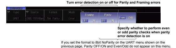
The DLM2000 triggers when it detects an error.
