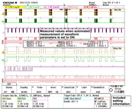
b. When ESC is pressed from the condition of a to hide the menu and the measured values of waveform parameters are displayed at the bottom of the screen
