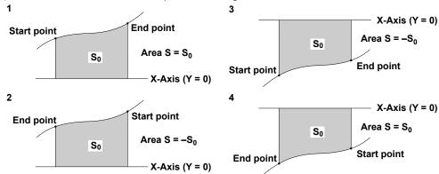
(2) When the Waveform Extends into the Negative Side
