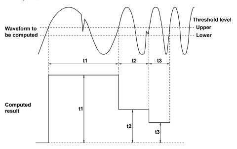
**Example 2, When the Interval Is Set to DUTYH**
