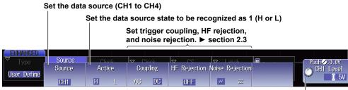
Set the level used to detect data source states
