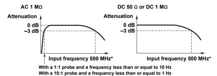
\* The high-frequency –3 dB point differs based on the model and the voltage scale settings.
