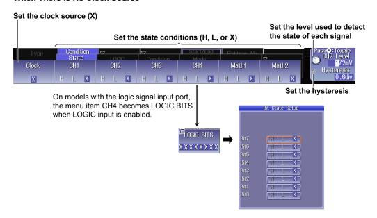
The same menu appears as that shown on the previous page for when the clock source is Math1, Math2, or from CH1 to CH4. Because there is no clock source, you can specify all of the signal states for Math1, Math2, from CH1 to CH4, and LOGIC as state conditions.
