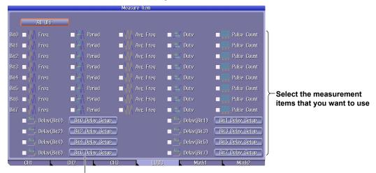
Configure the measurement of delay between waveforms
