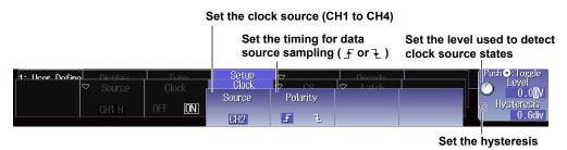
Specify which clock source edge causes the data source to be sampled.
