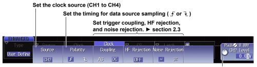
Set the level used to detect clock source states
