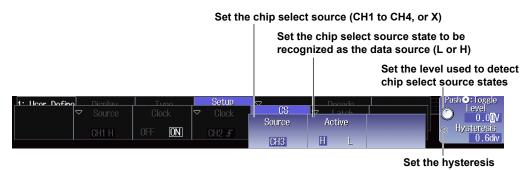
When the data source is sampled in sync with the clock source, use the chip select source to control the period for which the DLM2000 tests the data source.
