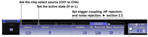
Set the level used to detect chip select source states
