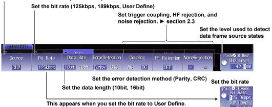
Set the level used to detect data frame source states
