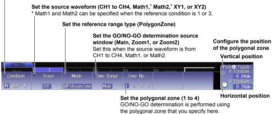
Use the Mask Editor software on a PC in advance to create the polygonal images that you will use as polygonal zones. After loading the file (see section 17.8) and loading the polygonal image into the specified zone number (Zone No. 1 to 4), configure the polygonal zone GO/NO-GO determination.
