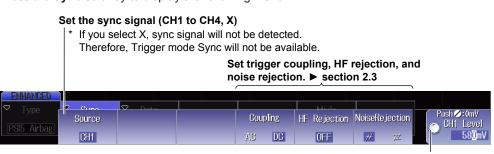
Set the level used to detect the state of the sync signal
