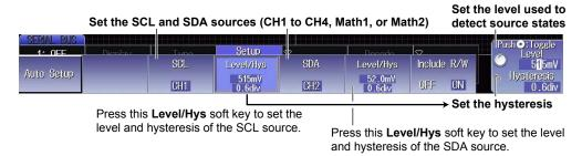
When the Source Is LOGIC (On models with the logic signal input port)
