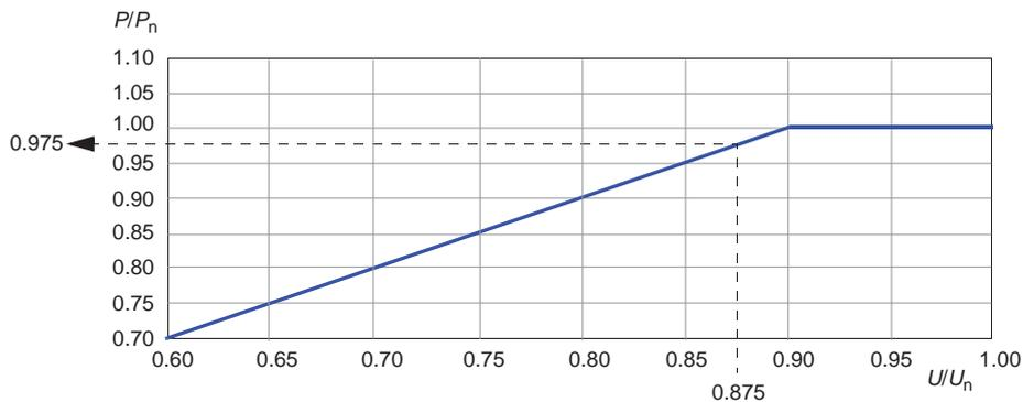
Example 1:  $P_n$  for ACS880-14-650A-3 is 355 kW. The input voltage ( $U$ ) is 350 V.  $\rightarrow U/U_n = 350 \text{ V} / 400 \text{ V} = 0.875$ .  $\rightarrow P/P_n = 0.975$   $\rightarrow$  The derated power  $P = 0.975 \times 355 \text{ kW} = 346 \text{ kW}$ .
