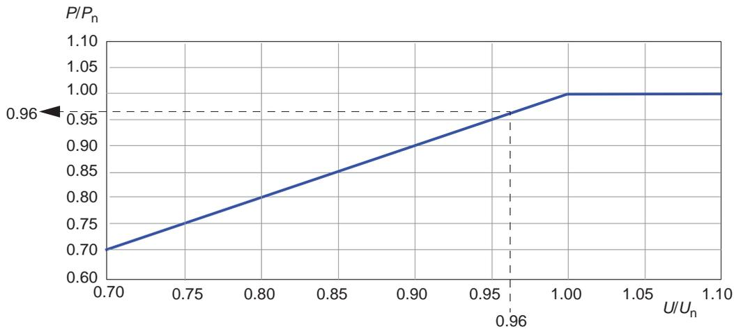
**Example 1:**  $P_n$  for ACS880-14-430A-7 is 400 kW. The input voltage ( $U$ ) is 660 V.  $\rightarrow U/U_n = 660 \text{ V} / 690 \text{ V} = 0.96 \rightarrow P/P_n = 0.96 \rightarrow$  The derated power  $P = 0.96 \times 400 \text{ kW} = 384 \text{ kW}$ .
