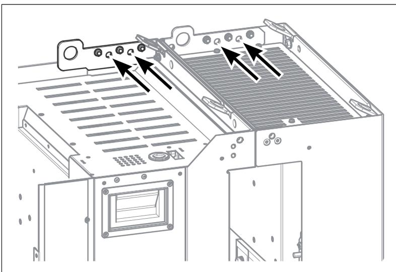
You can attach the modules to Rittal VX25 enclosure with the mounting brackets delivered with the drive, see [Step-by-step drawings for an installation example of standard drive configuration in Rittal VX25 800 mm wide enclosure \(page 233\)](#).
