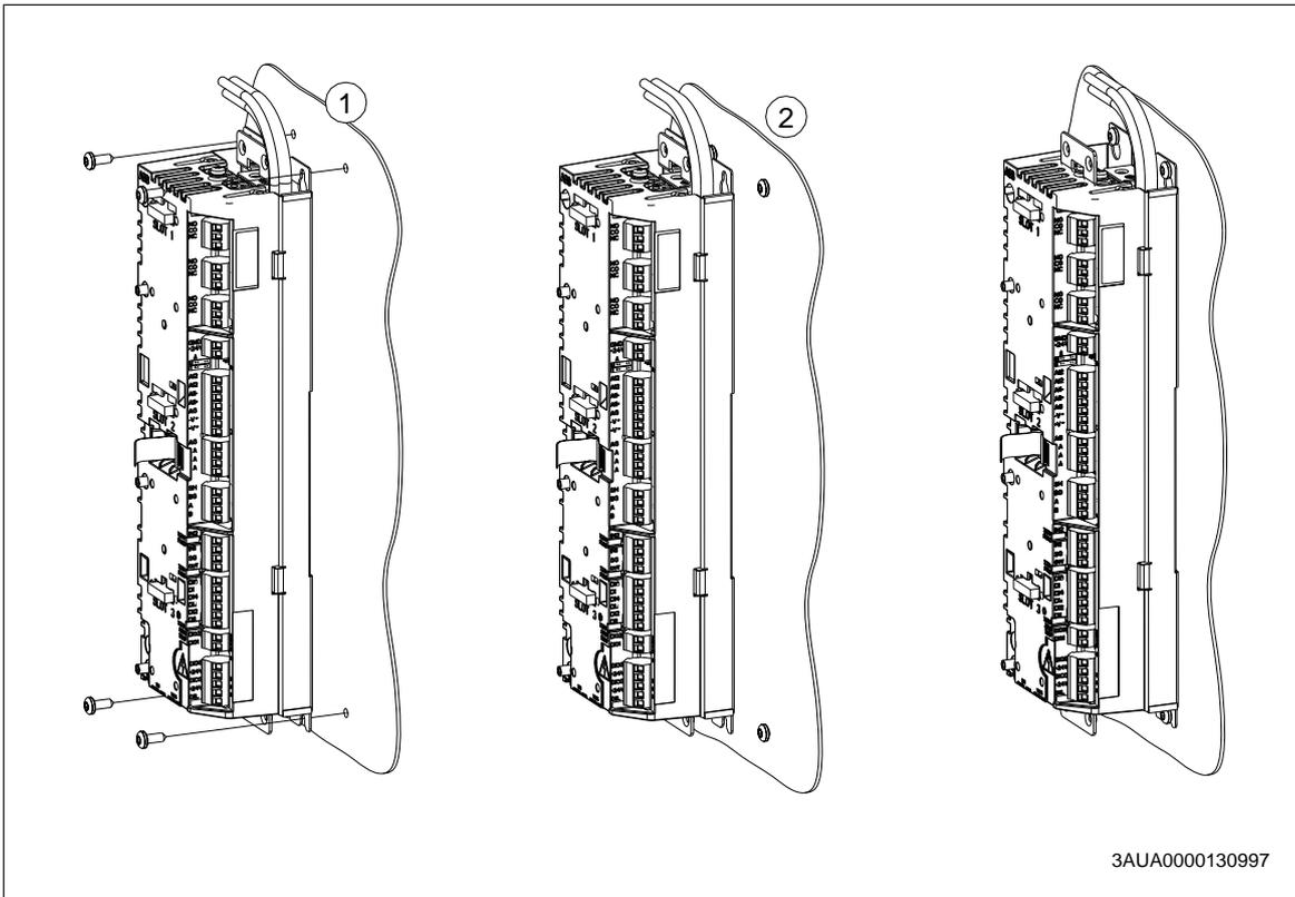
■ **Attaching the external control unit vertically on a DIN rail**
