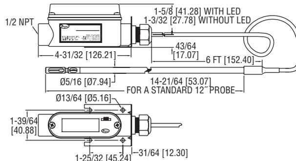
The **SERIES 641RM** features the same highly accurate heated mass flow sensor as the Series 641, with a remote probe construction. The units 6' cable which connects the sensing probe with the electronic enclosure allows the enclosure to be mounted where it can be more easily accessed.
