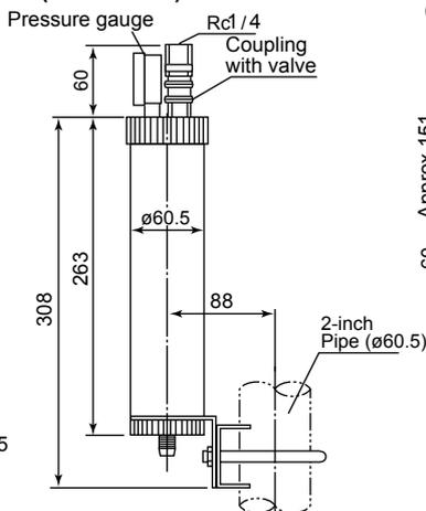
**Big volume tank KCl reserve tank for KCl filling pH sensor and pH sensor for high purity water. (with mounting bracket)**
