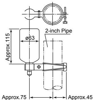
**Medium pressure KCl reserve tank for KCl filling pH/ORP sensor (with mounting bracket)**
