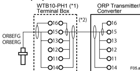
\*1: Terminal box is used only where pH transmitter/converter or ORP transmitter/converter is installed remotely from pH or ORP sensor (normally not needed).
