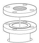
3. Tighten the bolts and nuts with sufficient torque for the flange and gasket choice.
