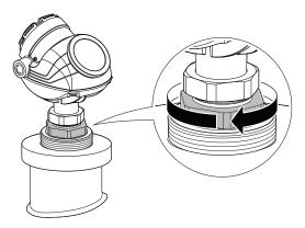
4. Rotate the transmitter head so the cable entries/display face the desired direction.
