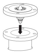
8. Fit the antenna onto the adapter and tighten the six M4 screws.
