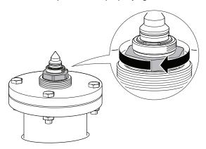
14. Mount the transmitter head and tighten the nut (torque 30 Lbft, 40 Nm).
