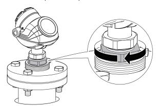
7. Rotate the transmitter head so the cable entries/display face the desired direction.
