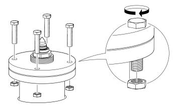
13. Screw the adapter until it is properly tightened.
