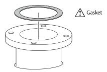
11. Lower the antenna and flange assembly into the tank.
