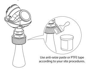
5. Lower the device into the tank.
