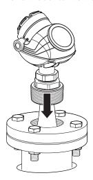
6. Screw the adapter into the process connection.
