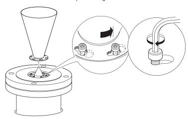
9. Carefully lift the antenna and flange assembly.
