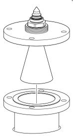
12. Tighten the bolts and nuts with sufficient torque for the flange and gasket choice.
