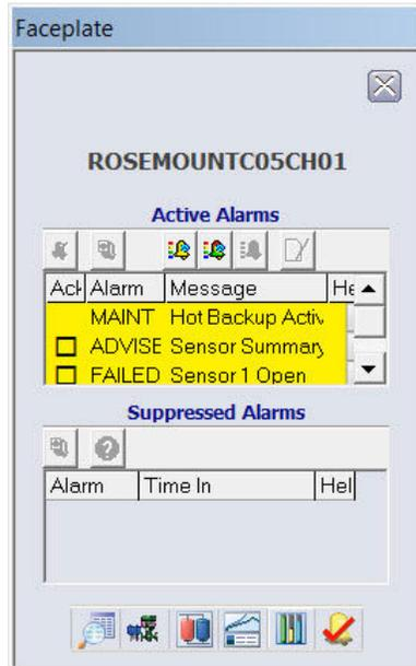
It is recommended that Hot Backup be reset immediately after repairing or replacing the affected sensor. See [Reset Hot Backup: Fast Keys 2-2-4-1-4](#). After resetting Hot Backup, the DeltaV Faceplate window indicates the alarms ADVISE Configuration Change and MAINTENANCE Hot Backup Active. You must acknowledge these alarms in order to clear them by checking the ACK boxes next to each alarm.
