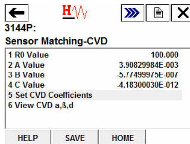
6. When prompted, select which set of coefficients you would like to enter for that sensor. Select between 1 R0, A, B, C and 2 R0, Alpha, Beta, Delta.
