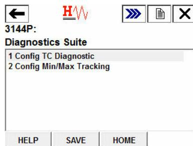
5. Select the sensor for which Thermocouple Diagnostic will be disabled. Select from 1 Sensor 1 or 2 Sensor 2 and select ENTER.
