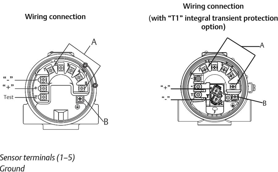
**Figure 2-12: Sensor Wiring Diagram for HART/4-20 mA**
