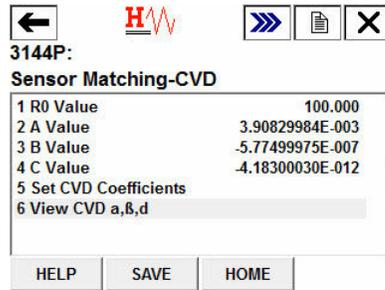
The following input constants, included with specially-ordered Rosemount temperature sensors, are required:
