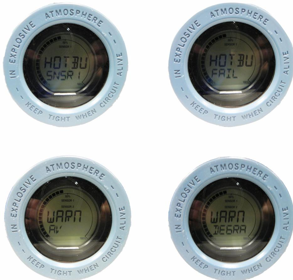
After the sensor has been repaired or replaced, the LCD display on the transmitter will display a message WARN HOT BU, reminding you that Hot Backup is still active, as well as the normal output of the average temperature. The warning message will clear after you have reset Hot Backup. It is recommended that Hot Backup be reset immediately after repairing or replacing the damaged sensor. See [Reset Hot Backup: Fast Keys 2-2-4-1-4](#).
