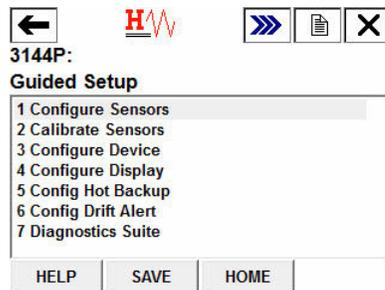
4. When prompted, select **1 Configure Sensor 1**. If you are using dual RTDs, you may also select **2 Configure Sensor 2**, or **3 Configure Both Sensors the Same**.
