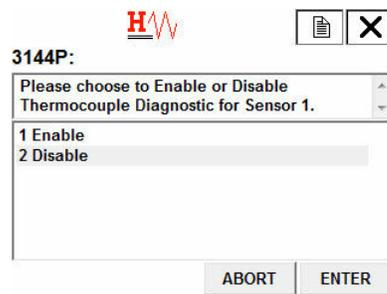
The screenshot shows a diagnostic screen with a red 'H' and a waveform icon at the top left. To the right are two icons: a document and an 'X'. Below the icon is the text '3144P:'. The main display area contains the text 'Please choose to Enable or Disable Thermocouple Diagnostic for Sensor 1.' followed by a list: '1 Enable' and '2 Disable'. At the bottom are two buttons: 'ABORT' and 'ENTER'.
