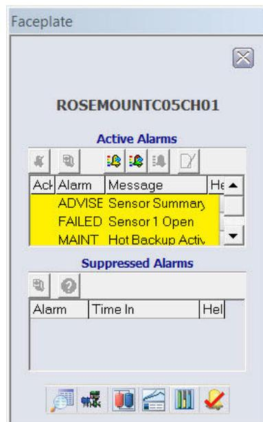
After the sensor has been repaired or replaced, the Faceplate window in DeltaV will display boxes next to each alarm that has been addressed. You must acknowledge each alarm to clear it by checking the ACK box to the left of the alarm.
