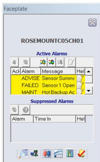
After the sensor has been repaired or replaced, the faceplate window in DeltaV will display boxes next to each alarm that has been addressed. You must acknowledge each alarm to clear it by checking the ACK box to the left of the alarm.
