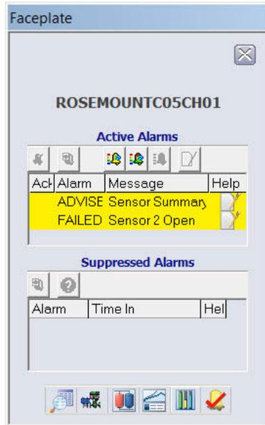
After the sensor has been repaired or replaced, the faceplate in DeltaV will display boxes next to the alarms, shown below. You must acknowledge these alarms by clicking on the boxes in order to clear them.
