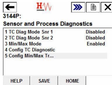
6. Select 1 Enable to enable the Min/Max Tracking feature and select ENTER.
