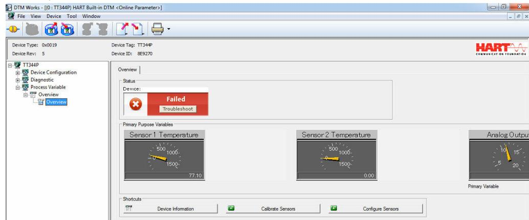
To investigate why the device displays a Failed status, select **Troubleshoot** in the red device status box. Another screen will display the active alerts indicating FAILED Sensor 2 Open, as shown below:
