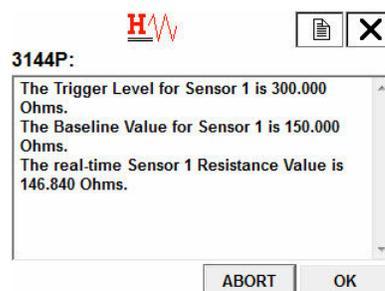
The screenshot shows the same HART communicator interface as in step 9. The main display area shows the same summary: 'The Trigger Level for Sensor 1 is 300.000 Ohms.', 'The Baseline Value for Sensor 1 is 150.000 Ohms.', and 'The real-time Sensor 1 Resistance Value is 146.840 Ohms.'. At the bottom of the screen are two buttons: 'ABORT' and 'OK'.
