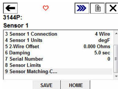
5. The screen would display a summary screen of the coefficients  $R_0$ ,  $A$ ,  $B$ , and  $C$ . Select 6 View CVD  $\alpha$ ,  $\beta$ ,  $\delta$  to view those.
