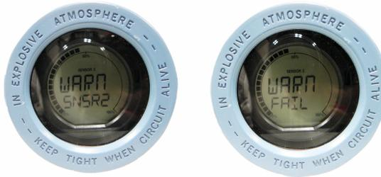
After the sensor has been repaired or replaced, the LCD display warning message will clear and display the output of the primary variable.
