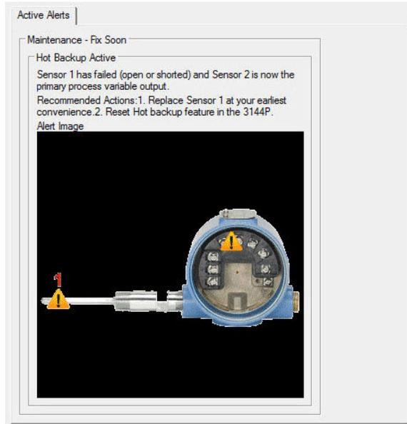
It is recommended that Hot Backup be reset immediately after repairing or replacing the affected sensor. See [Reset Hot Backup: Fast Keys 2-2-4-1-4](#) with a Field Communicator or reset it directly in the DTM by going to the Diagnostics tab of the Manual Setup section and selecting **Reset Hot Backup**, as shown below:
