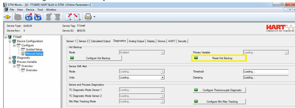
After resetting Hot Backup, the device status in the Process Variable Overview section of the DTM will change from Maintenance to Advisory, as shown below:
