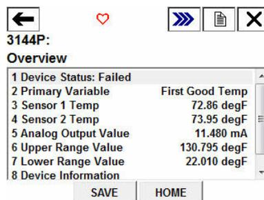
If Sensor Drift Alert is configured in Warning Mode, select 1 Device Status: Maintenance.
