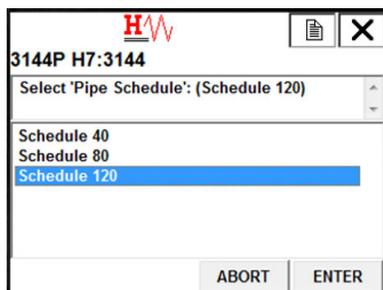
5. If process *Pipe Material*, *Line Size*, or *Pipe Schedule* is not available under Rosemount X-well Process selection, select **Rosemount X-well Custom** sensor type.
