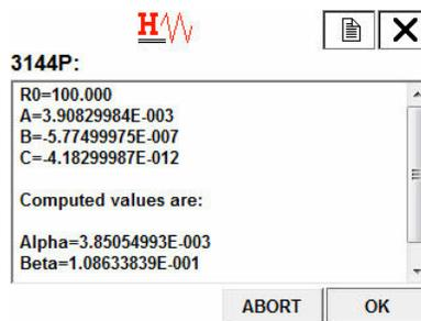
11. Finish the remaining steps of the sensor configuration according to the Communicator. When you are satisfied with your selection, select 6 Exit from the main screen, or select Abort.
