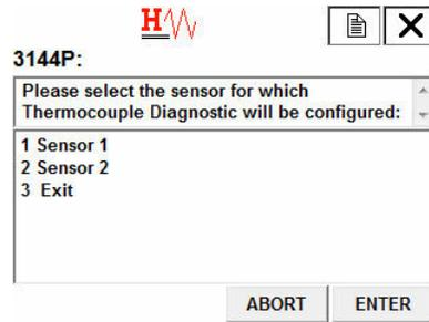
The screenshot shows a diagnostic screen with a red 'H' and a waveform icon at the top left. To the right are two icons: a document and an 'X'. Below the icon is the text '3144P:'. The main display area contains the text 'Please select the sensor for which Thermocouple Diagnostic will be configured:' followed by a list: '1 Sensor 1', '2 Sensor 2', and '3 Exit'. At the bottom are two buttons: 'ABORT' and 'ENTER'.
