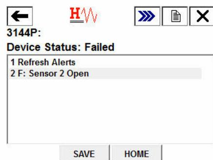
After the sensor has been repaired or replaced, the Field Communicator will display a Good Device Status, indicating the problem is solved.
