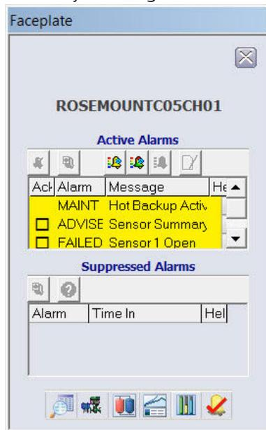
It is recommended Hot Backup be reset immediately after repairing or replacing the affected sensor. See “Reset Hot Backup: Fast Keys 2-2-4-1-4” on page 76. After resetting Hot Backup, the DeltaV Faceplate window indicates the alarms *ADVISE Configuration Change* and *MAINTENANCE Hot Backup Active*. You must acknowledge these alarms in order to clear them by checking the *ACK* boxes next to each alarm.
