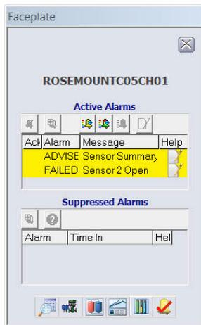
After the sensor has been repaired or replaced, the faceplate in DeltaV will display boxes next to the alarms, shown below. You must acknowledge these alarms by clicking on the boxes in order to clear them.
