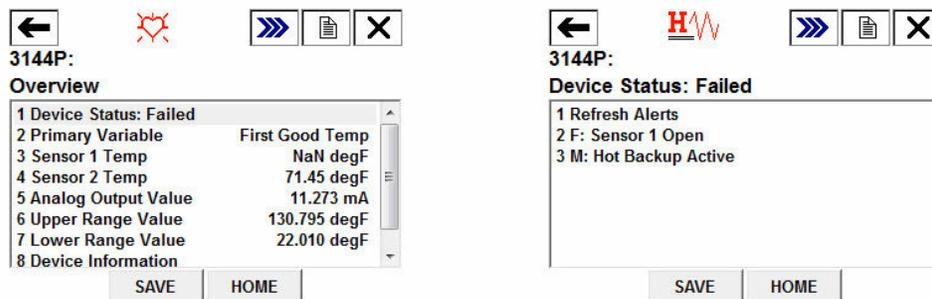
After the sensor has been repaired or replaced, the Field Communicator will display a maintenance device status, indicating Hot Backup is still active. This is shown in the Field Communicator in the Overview section.
