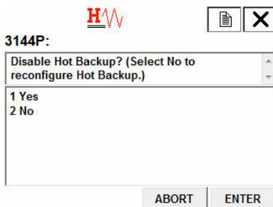
5. When prompted, choose which variable you would like as your primary variable (PV) and select ENTER. With Hot Backup disabled, the PV may be *Sensor 1 Temperature*, *Sensor 2 Temperature*, *Differential Temperature*, *Average Temperature*, or *First Good Temperature*.
