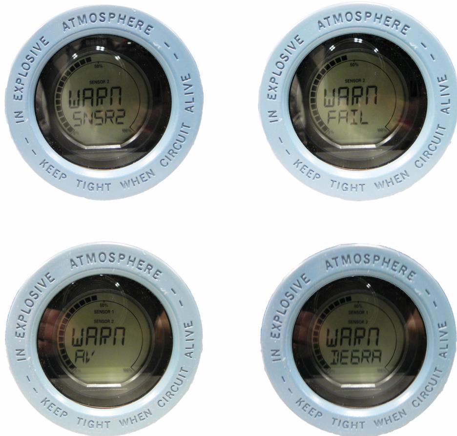
After the sensor has been repaired or replaced, the LCD display warning message will clear and display the output of the primary variable.
