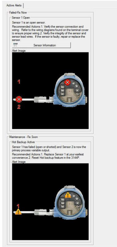
After the sensor has been repaired or replaced, the device status in the Process Variable Overview section of the DTM will change from Failed to Maintenance.
