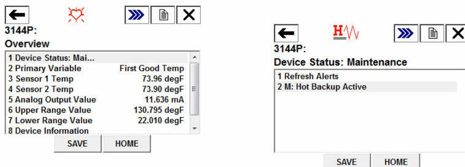
It is recommended Hot Backup be reset immediately after repairing or replacing the affected sensor. See [Reset Hot Backup: Fast Keys 2-2-4-1-4](#). After resetting Hot Backup, the Field Communicator will display an Advisory Device Status, indicating that the configuration has changed. This is shown in the *Overview* section. To clear this advisory, clear the configuration changed flag, as shown below:
