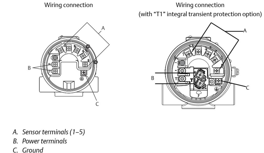
Figure 2-15: Sensor Wiring Diagram for FOUNDATION Fieldbus
