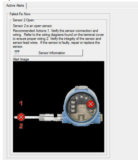
After the sensor has been repaired or replaced, the alerts will clear, and the yellow circles in the PRM change to green, indicating that everything is operating correctly. Hot Backup does not need to be reset in this case.
