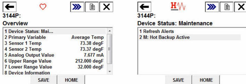
It is recommended that Hot Backup be reset immediately after repairing or replacing the affected sensor. See [Reset Hot Backup: Fast Keys 2-2-4-1-4](#). After resetting Hot Backup, the Field Communicator will display an Advisory Device Status, indicating that the configuration has changed. This is shown in the Overview section. To clear this advisory, simply clear the configuration changed flag, as shown below:
