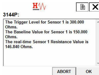
The screenshot shows the same HART communicator interface. The main display area now shows a summary: 'The Trigger Level for Sensor 1 is 300.000 Ohms.', 'The Baseline Value for Sensor 1 is 150.000 Ohms.', and 'The real-time Sensor 1 Resistance Value is 146.840 Ohms.'. At the bottom of the screen are two buttons: 'ABORT' and 'OK'.
