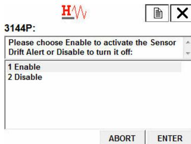
5. When prompted, select whether you want Sensor Drift Alert to put the transmitter into “Alarm” or “Warning”, and select ENTER. Enabling drift alert option warning only will set a flag (through HART Protocol) whenever the maximum acceptable difference between Sensor 1 and Sensor 2 has been exceeded. Enabling drift alert option alarm will send the transmitter's analog signal into alarm when drift alert is detected.
