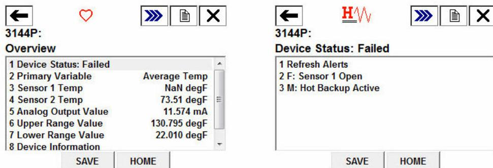
After the sensor has been repaired or replaced, the Field Communicator will display a Maintenance Device Status, indicating Hot Backup is still active. This is shown on the Field Communicator in the *Overview* section.
