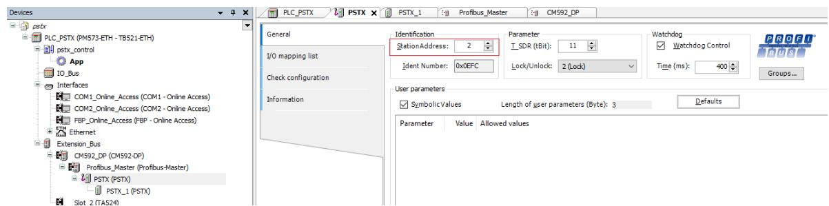
5. Map the signals to variable names in DP-Module I/O Mapping for the object PSTX\_1.
