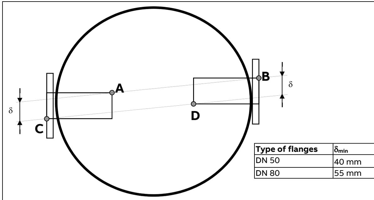
Figure 2-4: Flange line-up tolerances
