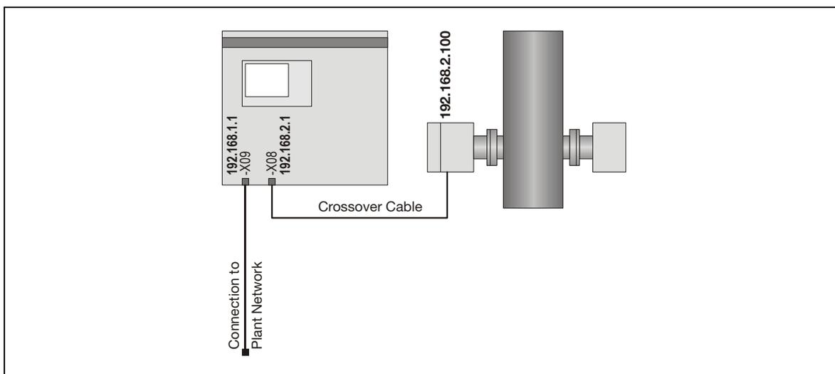
Figure 6-4: Ethernet connection – AO2000 with one laser analyzer
