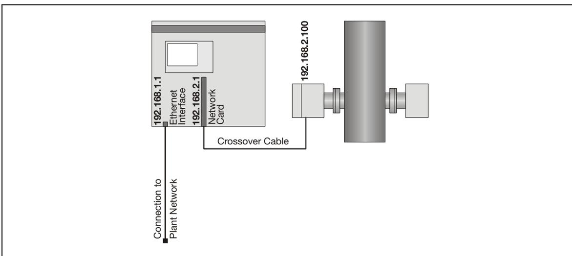
Figure 6-2: Ethernet connection – AO2000 with one laser analyzer
