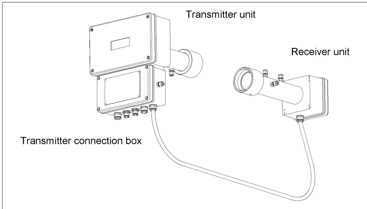
Figure 9-1: AO2000-LS25 for installation in ATEX Zone 2
