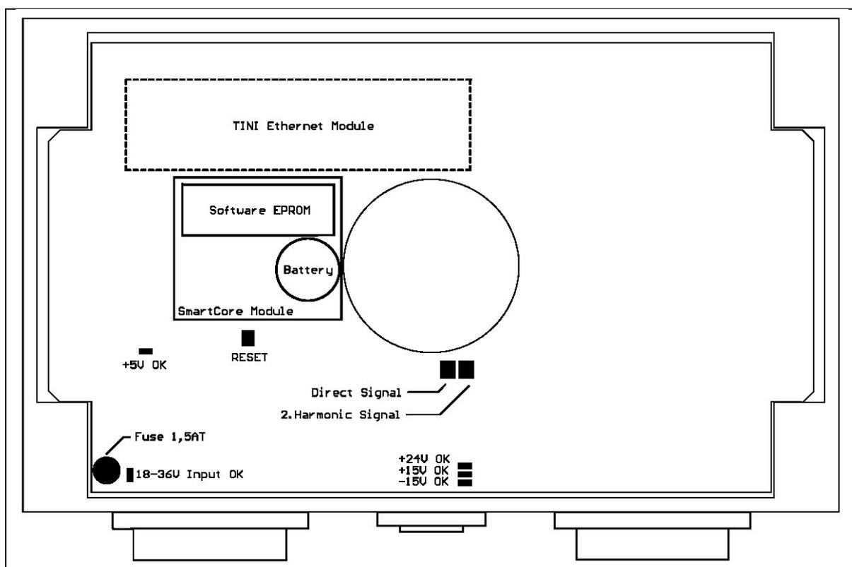
Figure 6-8: Power electronics card fuses and LED's layout
