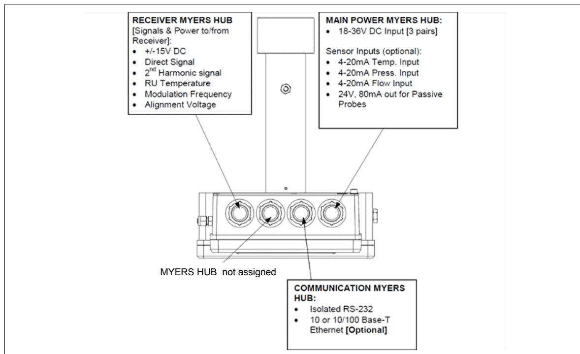
Figure 8-2: Transmitter unit – electronic interface
