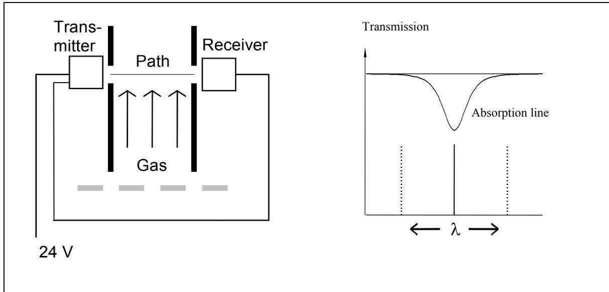
Figure 1-1: Measuring principle AO2000-LS25
