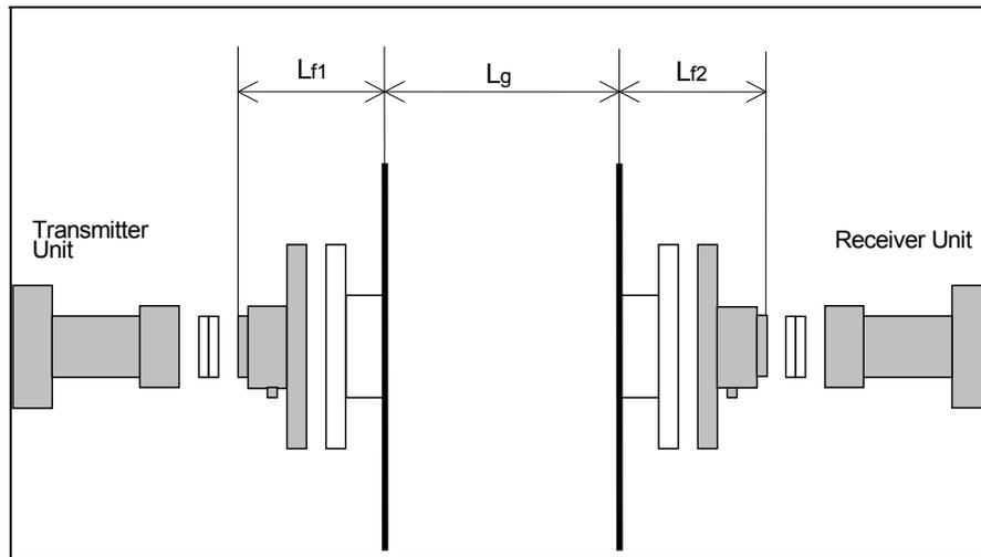
Figure 4-1: Optical lengths needed for setting initial parameters
