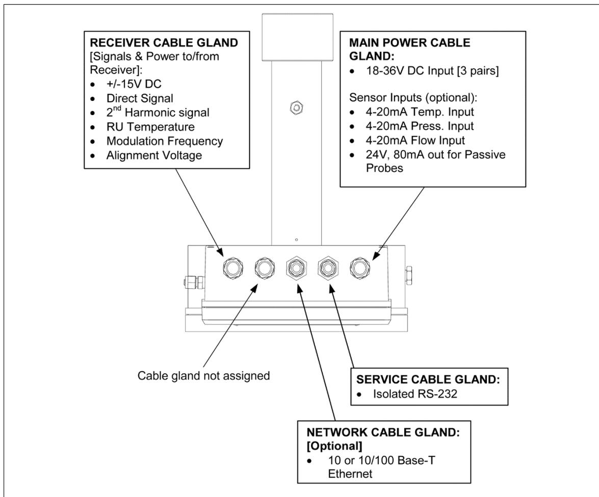
Figure 9-2: Transmitter unit – electronic interface
