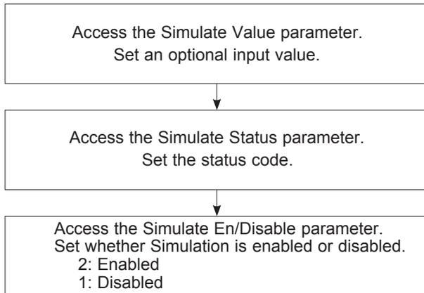
If simulation is enabled, AI block uses Simulate Status and Simulate Value as the input, and if disabled, the AI block uses Transducer Status and Transducer Value as input.
