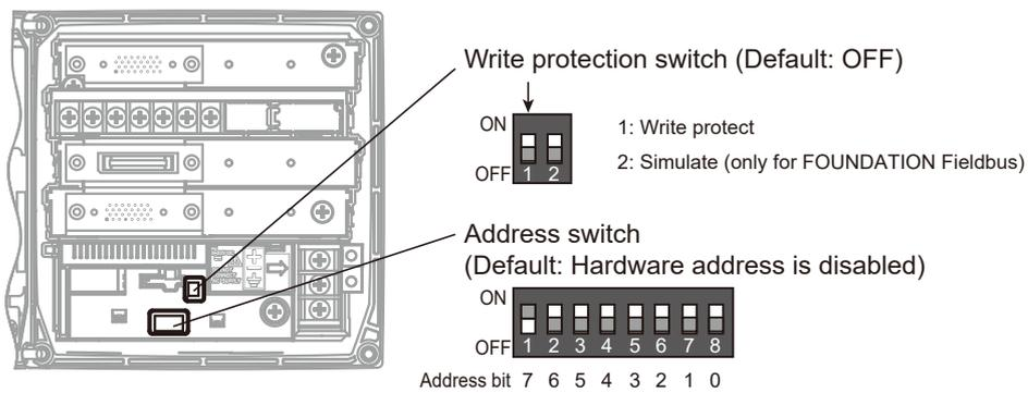
Figure 2.3 DIP switches
