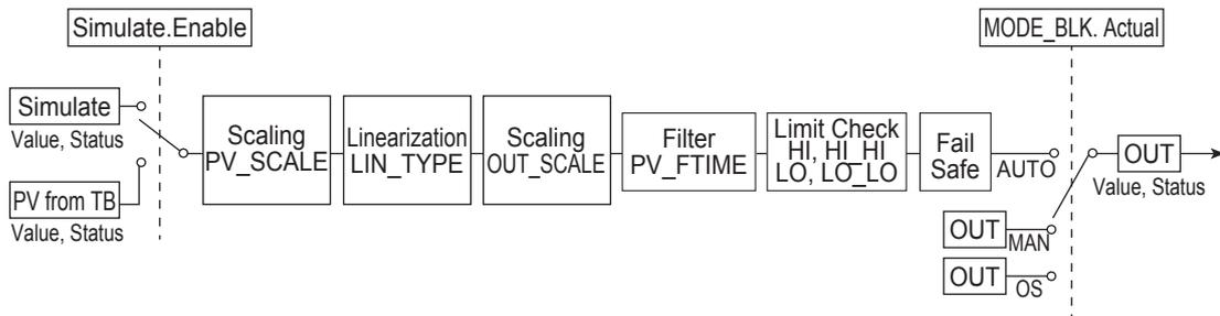
Figure 4.1 Diagram of the AI Functional Block
