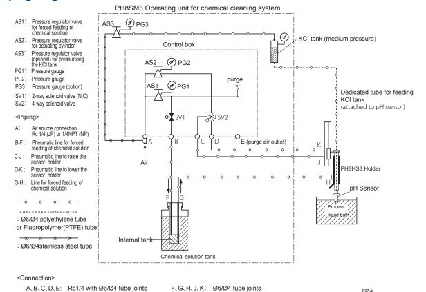
Note 1: For the piping between the cleaning unit and the sensor holder, a 40 m tube including joints are provided with the product Cut the tube to required length for use. The maximum length is 10 m to pipe between the cleaning unit and the sensor. Note 2: The tubes and joints are made of polyethylene resin or Fluoropolymer (PTFE). They should be replaced approximately once a year, although the intervals may vary depending on the chemicals used.
