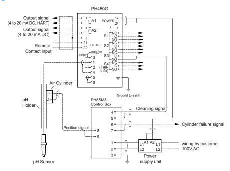
Electrical connections on the control box : Watertight plastic gland equivalent to JIS A15 (outside diameter : 9 to 12mm)
