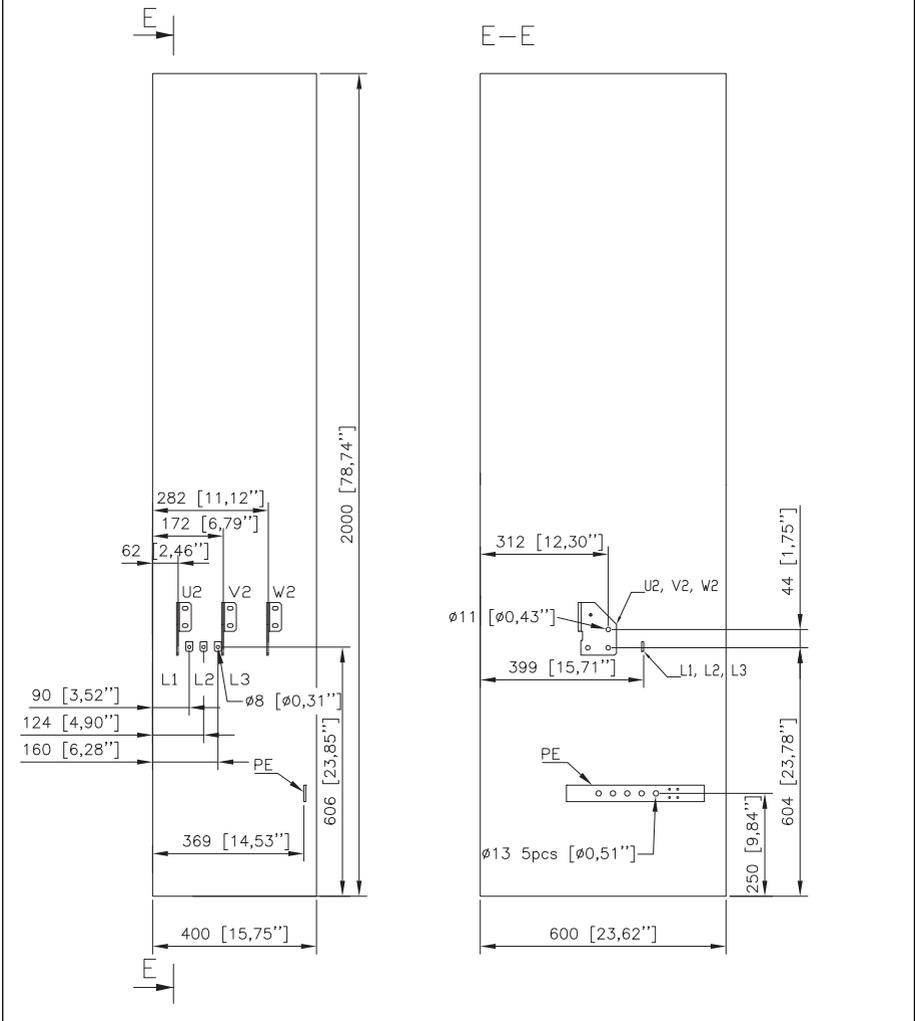
Frame R7: Input and motor cable terminal dimensions (bottom entry and exit, switch fuse OS250)
