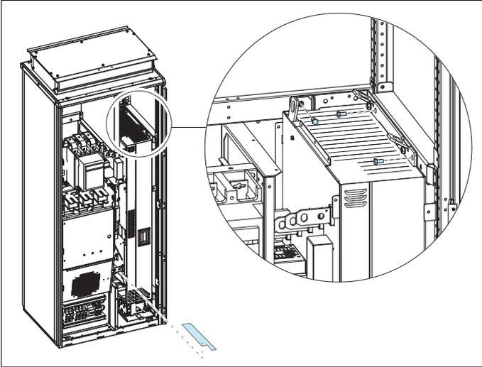
10. Attach the extraction ramp to the cabinet base with two screws.
