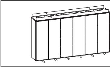
Lay the cabinet on the rollers and move it carefully until close to its final location. Remove the rollers by lifting the unit with a crane, forklift, pallet truck or jack.
