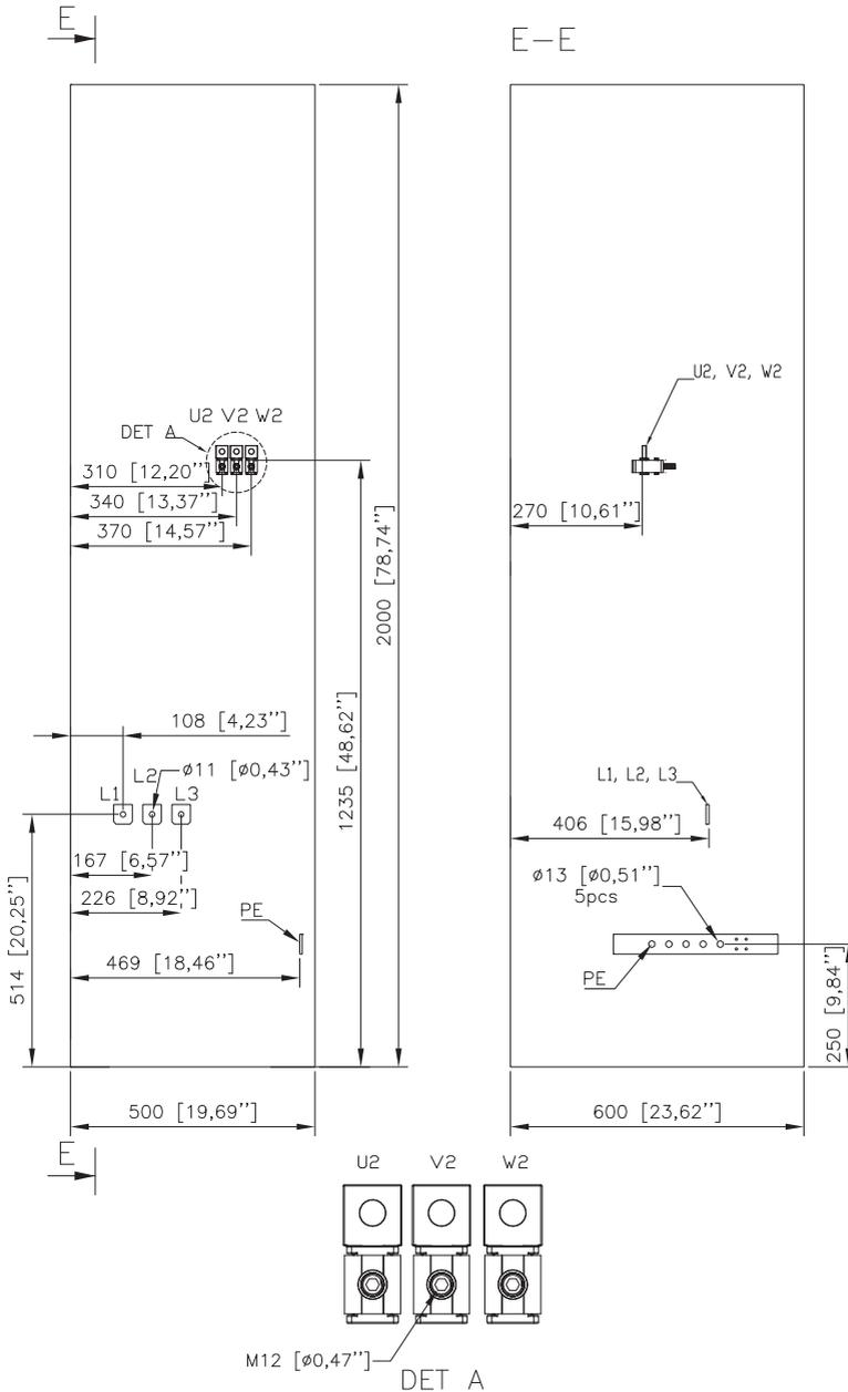
Frame R9: Input and motor cable terminal dimensions (bottom entry and exit, switch-disconnector OT630, du/dt filter [option +E205])
