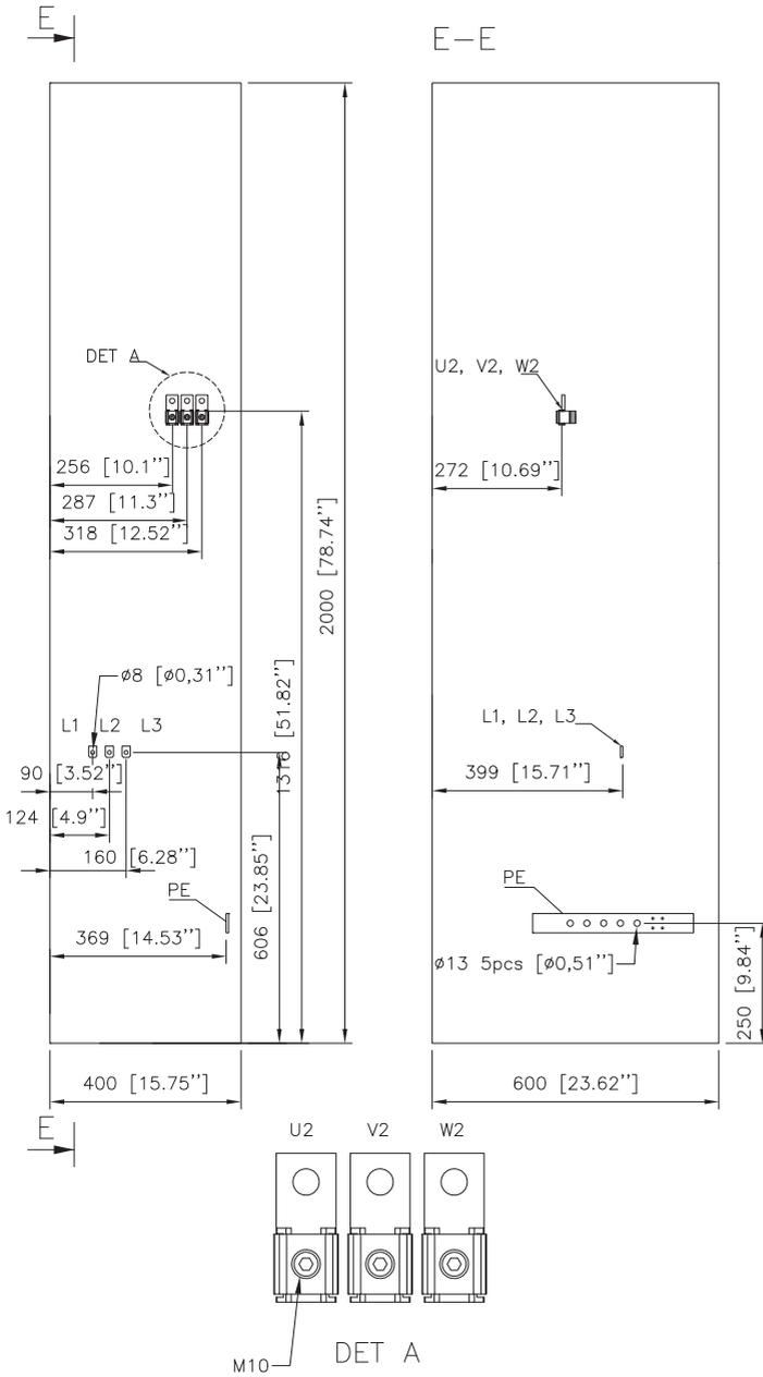
Frame R8: Input and motor cable terminal dimensions (bottom entry and exit, switch-disconnector OT400)
