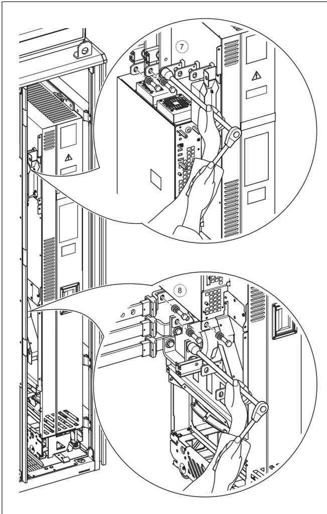
9. Remove the shroud. Undo the screws that attach the drive module to the cabinet at the top and behind the front support legs.
