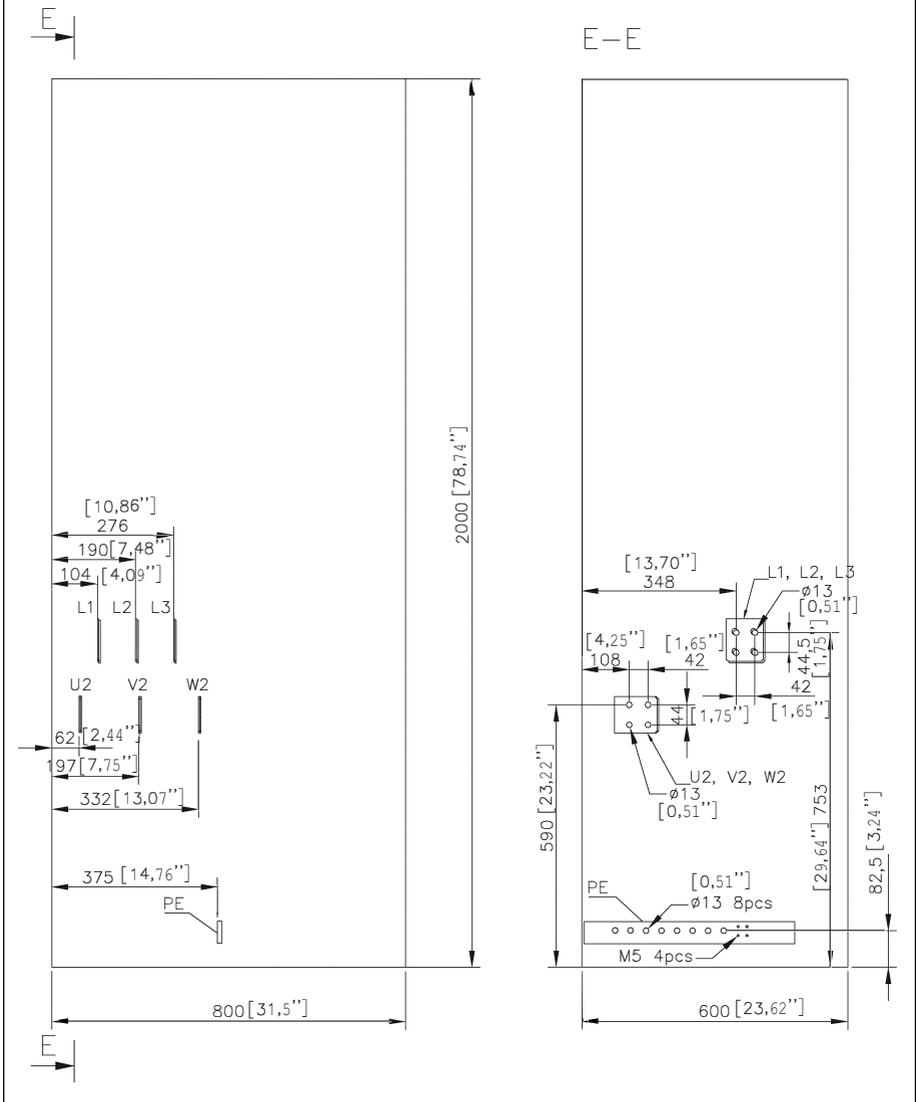
Frame R11: Input and motor cable terminal dimensions (top entry and exit)
