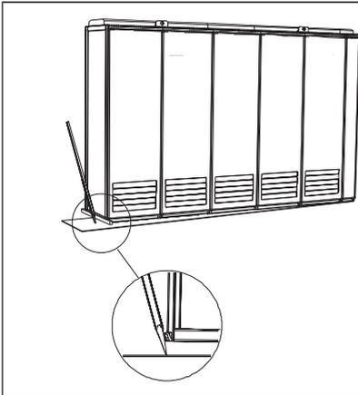
Move the cabinet into its final position with an iron bar. Place a wooden piece at the bottom edge of the cabinet in order not to damage the cabinet frame with the iron bar.
