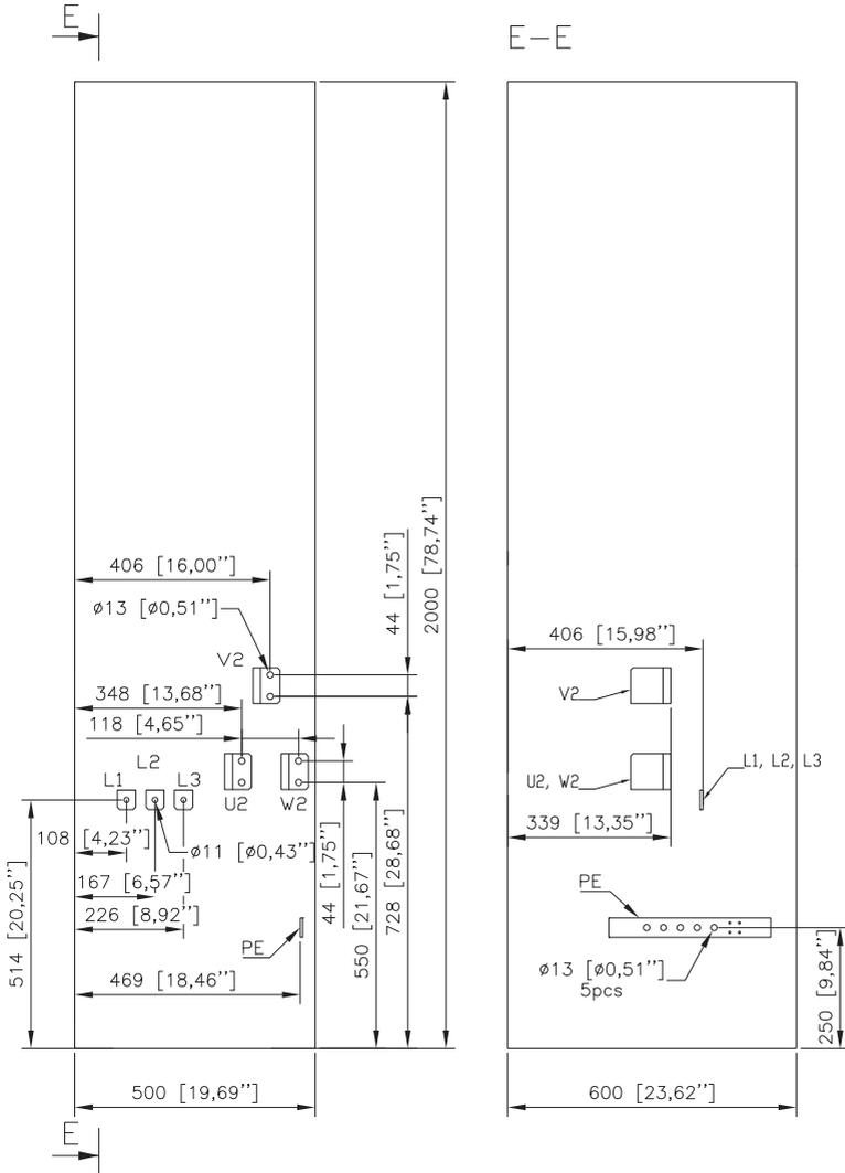
Frame R9: Input and motor cable terminal dimensions (option +F289)
