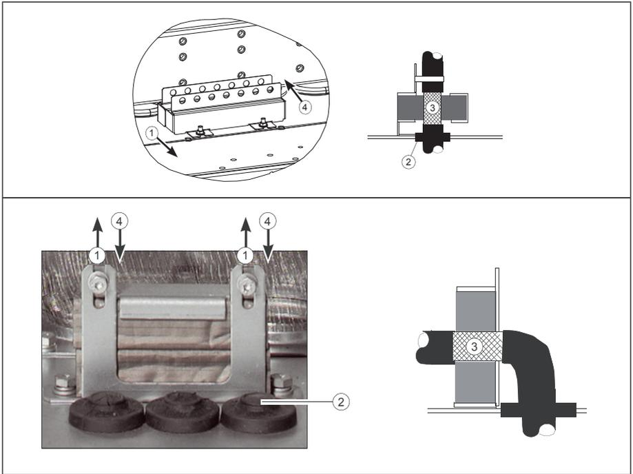
**Note 1:** Keep the shields continuous as close to the connection terminals as possible. Secure the cables mechanically at the entry strain relief.
