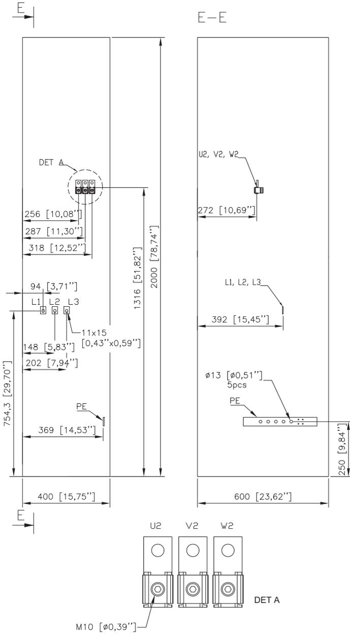
Frame R7: Input and motor cable terminal dimensions (bottom entry and exit, switch fuse OS400)
