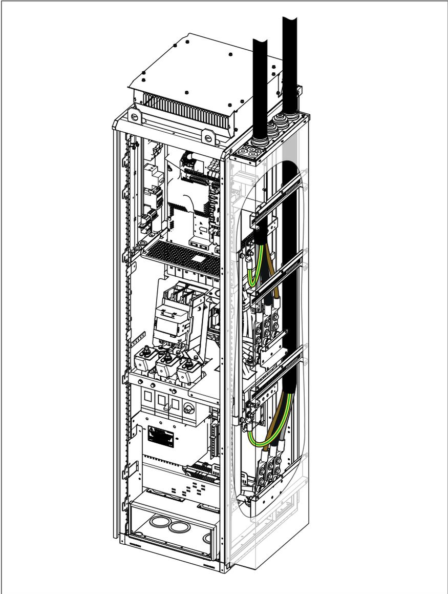
6. Tighten the power cable screws to the torque given in *Terminal and entry data for the power cables (page 209)*.
