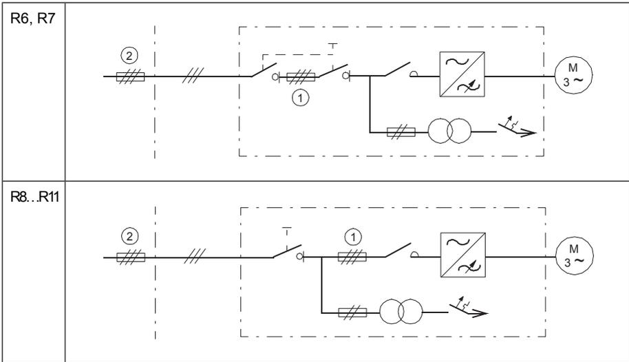
■ **Protecting the motor and motor cable in short-circuits**
