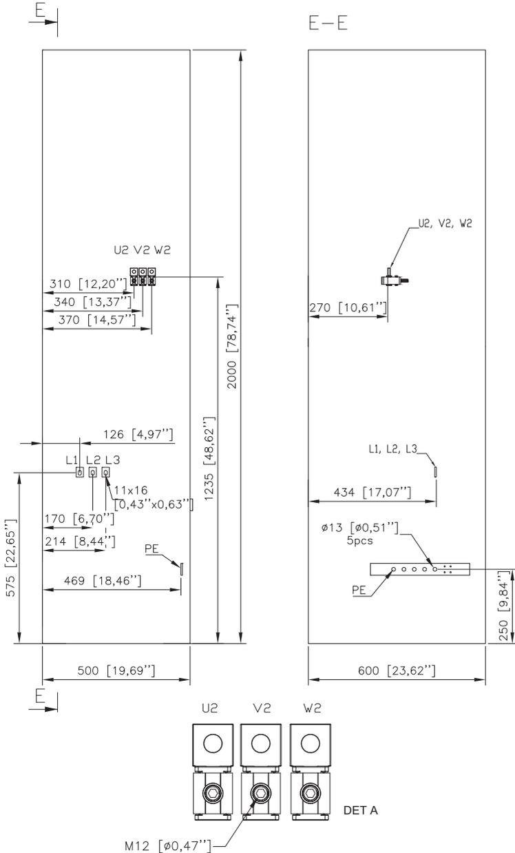
Frame R8: Input and motor cable terminal dimensions (bottom entry and exit, switch-disconnector OT400, du/dt filter [option +E205])
