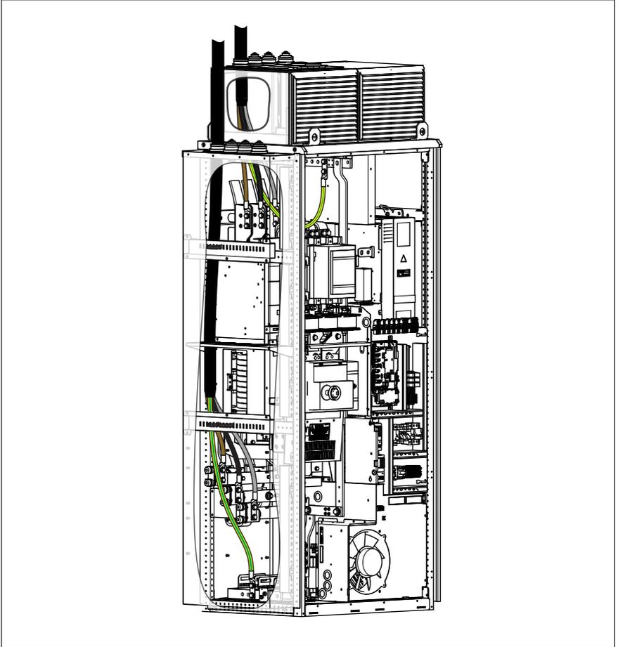
7. Tighten the power cable screws to the torque given in [Terminal and entry data for the power cables \(page 209\)](#).
