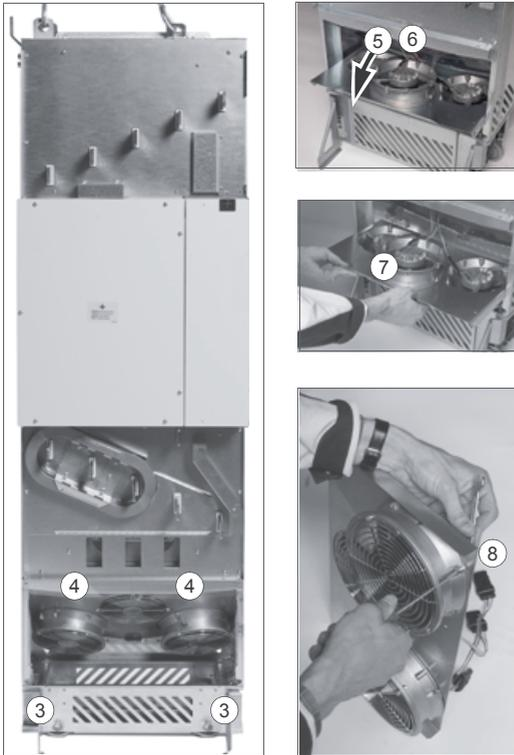
■ Replacing the auxiliary cooling fan of the drive module (frames R6...R9)
