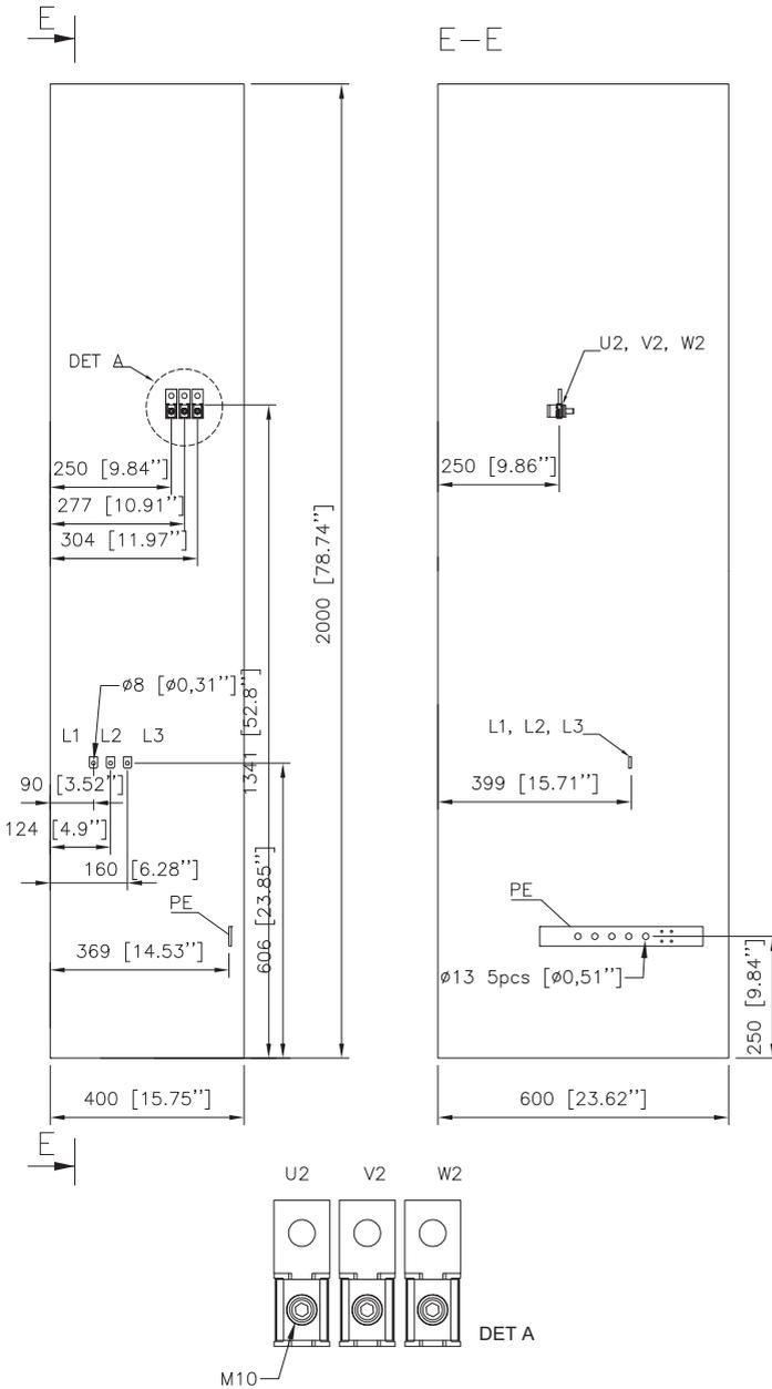
Frames R6 and R7: Input and motor cable terminal dimensions (bottom entry and exit, switch fuse OS250, du/dt filter [option +E205])
