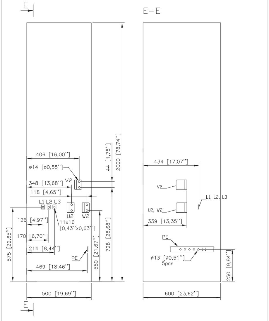
Frame R8: Input and motor cable terminal dimensions (bottom entry and exit, option +F289)
