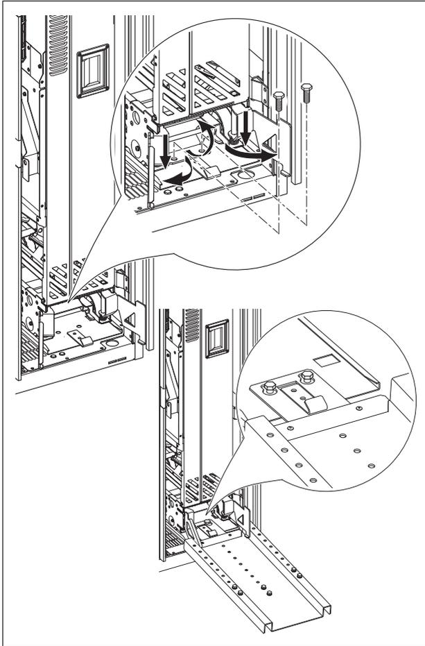
11. Attach the drive module lifting lugs to the cabinet lifting lug with chains.
