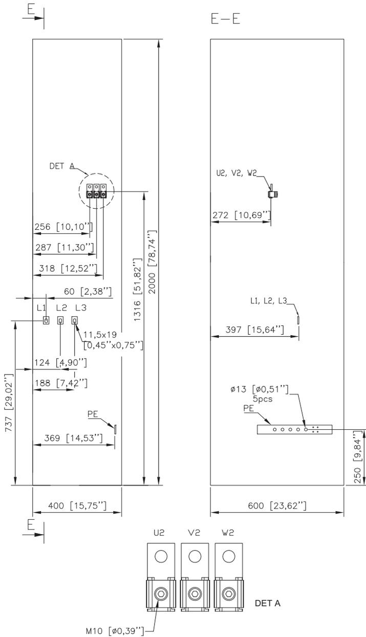
Frame R7: Input and motor cable terminal dimensions (bottom entry and exit, option +F289)
