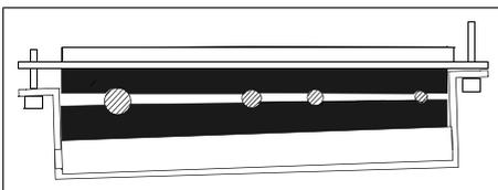
6. If more than one cable go through a grommet, seal the grommet by applying Loctite 5221 inside the grommet.
