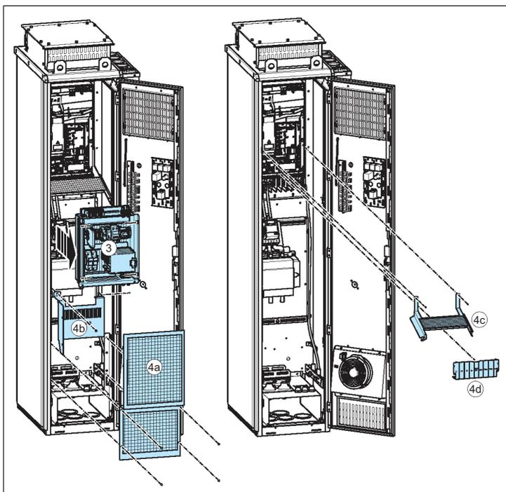
5. For drives without option +E205: Knock out holes in the shroud for the motor cable conductors.
