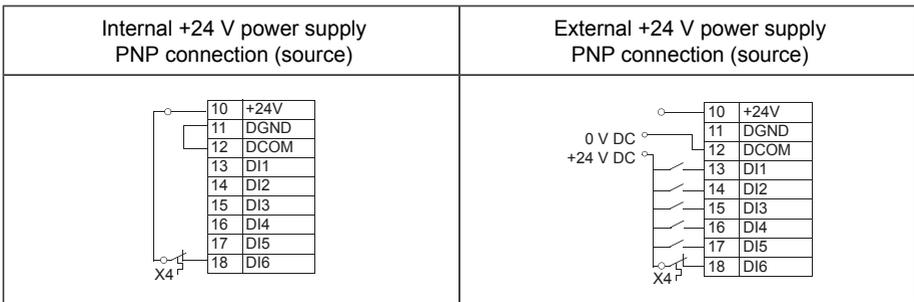
**⚡ WARNING!** Do not connect the +24 V AC cable to the control board ground when the control board is powered using an external 24 V AC supply.
