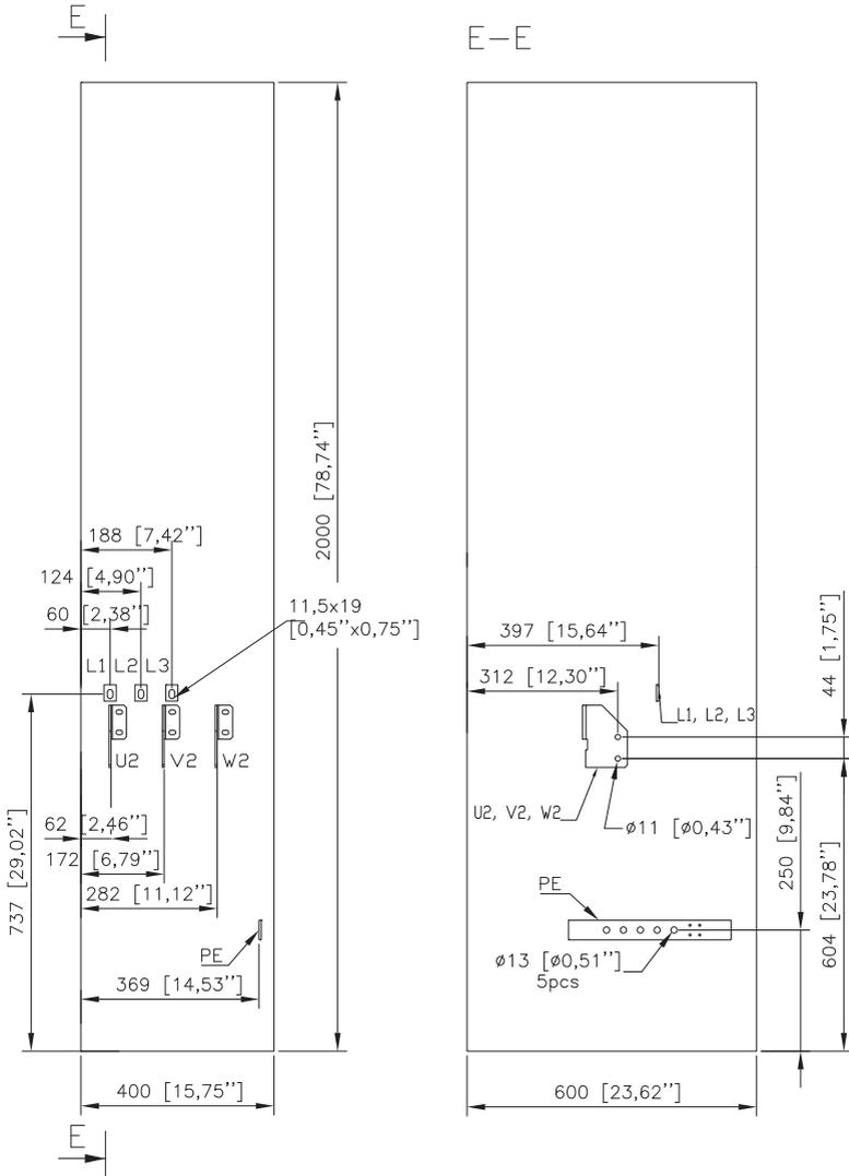
Frames R6 and R7: Input and motor cable terminal dimensions (bottom entry and exit, options +F289 and +E205)
