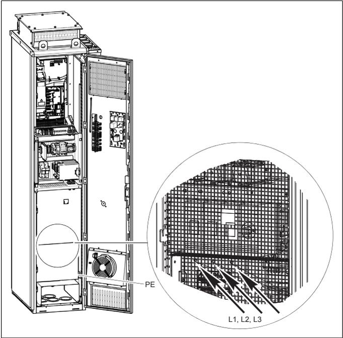
Measuring points of frames R10 and R11 are shown below. You can also remove the metallic shield and measure through the holes in the clear plastic shroud behind it.
