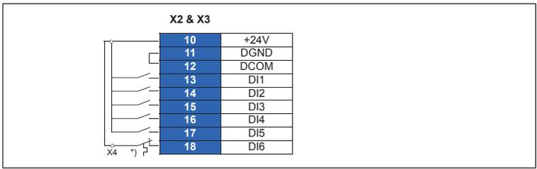
\*) Internal overtemperature supervision of the cabinet is connected between DI6 and +24V auxiliary voltage supply.
