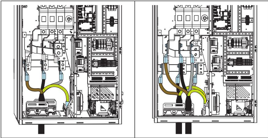
7. Tighten the power cable screws to the torque given in *Terminal and entry data for the power cables (page 209)*.
