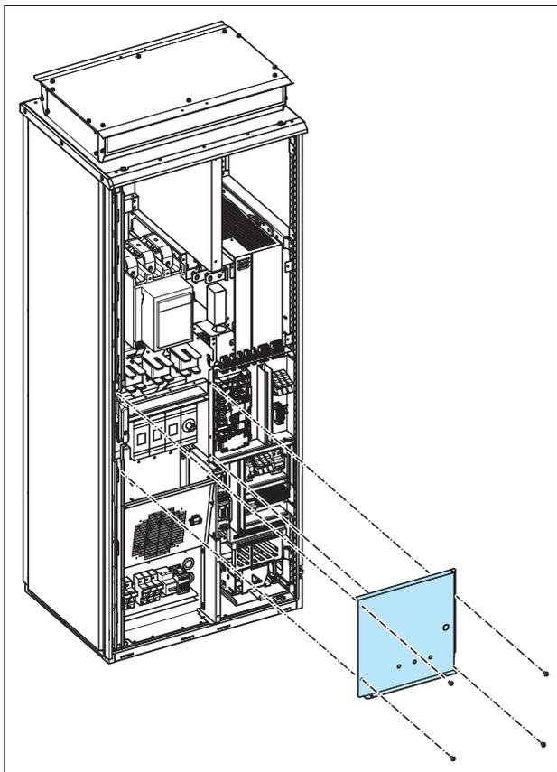
4. Remove the door fan mounting plate. See section *Replacing the door fan (frames R10 and R11) (page 166)*
