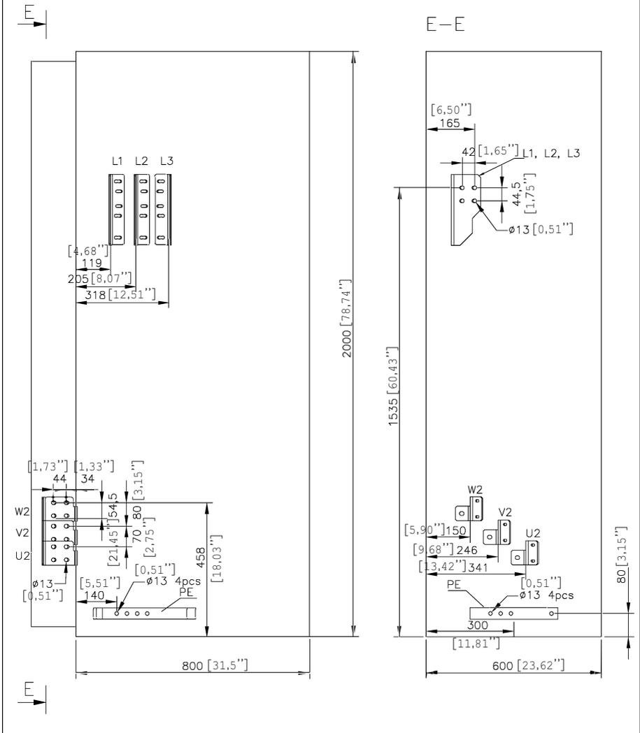
Frame R10: Input and motor cable terminal dimensions (top entry and exit, option +F289)
