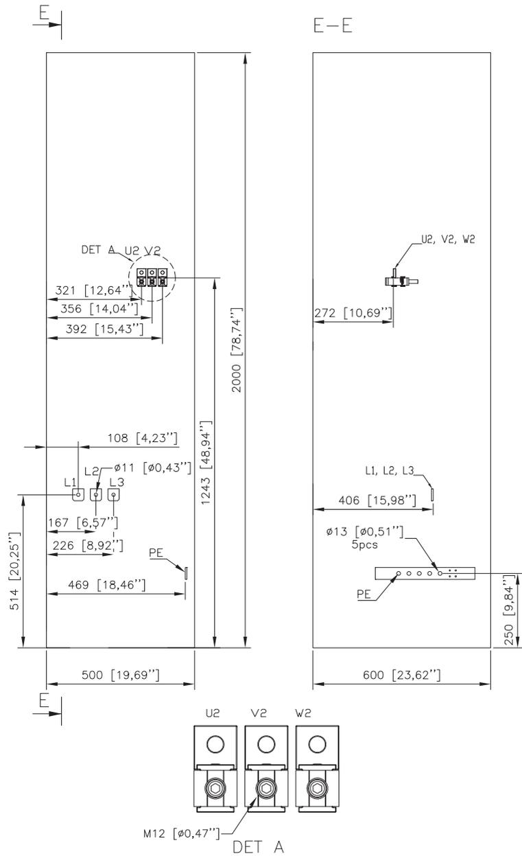
Frame R10: Input and motor cable terminal dimensions (top entry and exit)
