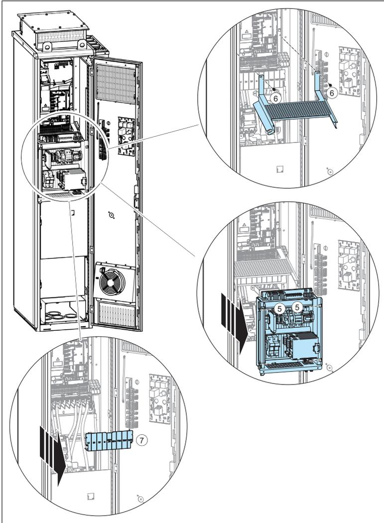
8. Disconnect the option modules from the control unit.
