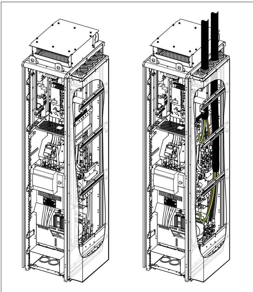
6. Tighten the power cable screws to the torque given in *Terminal and entry data for the power cables (page 209)*.
