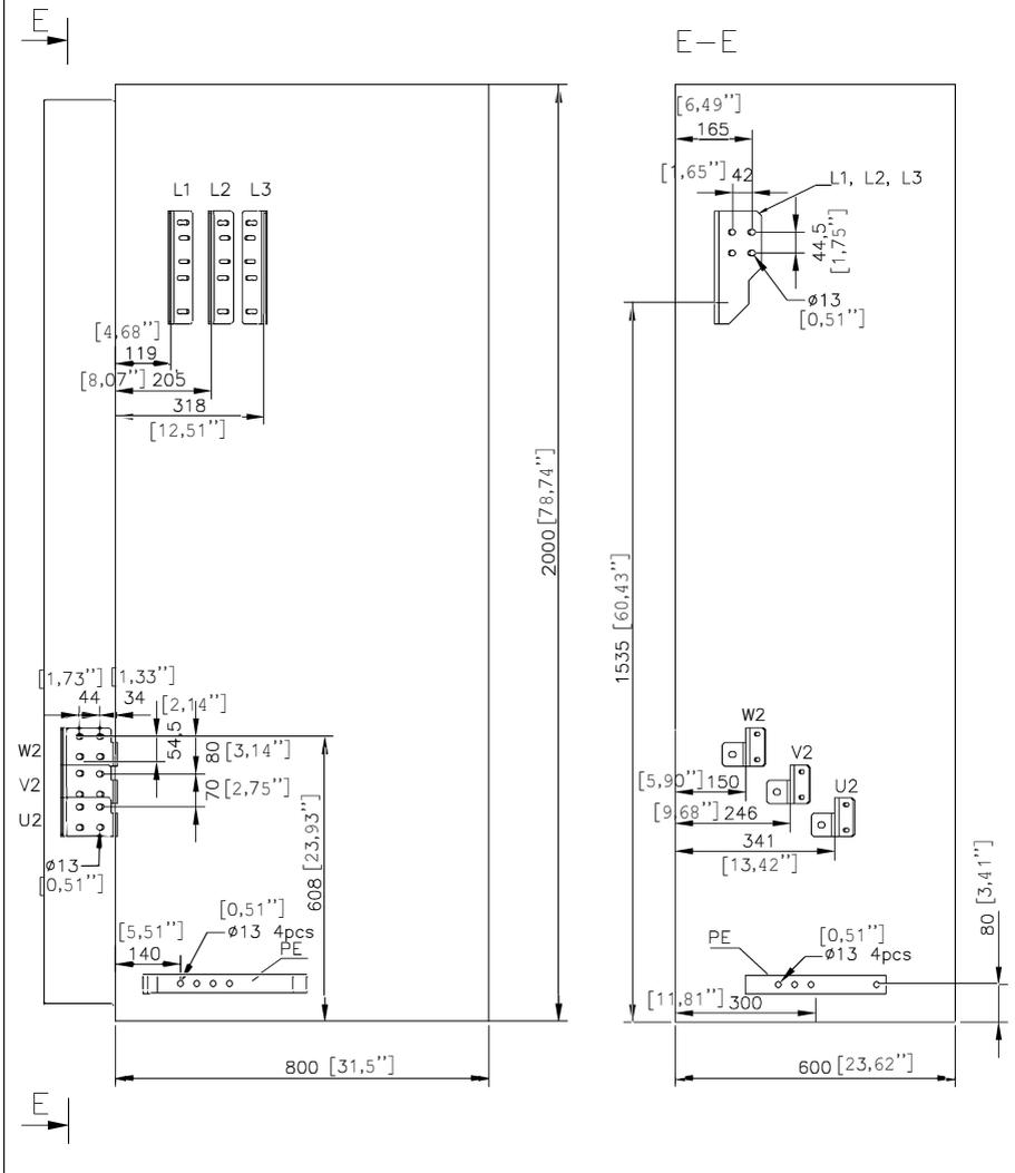
Frame R11: Input and motor cable terminal dimensions (top entry and exit, option +F289)
