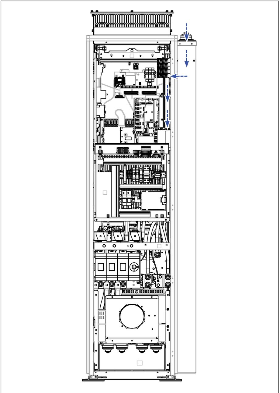
The route of the control cables for frames R10 and R11 is shown below.
