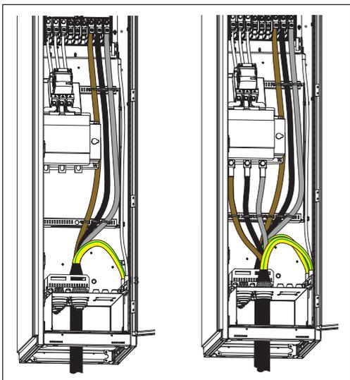
8. Tighten the power cable screws to the torque given in *Terminal and entry data for the power cables (page 209)*.
