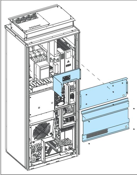
Remove the door fan mounting plate. See section *Replacing the door fan (frames R10 and R11) (page 166)*
