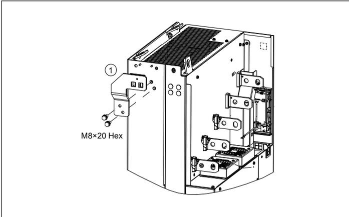
2. Install the telescopic extraction and insertion ramp to the cabinet base with two screws.
