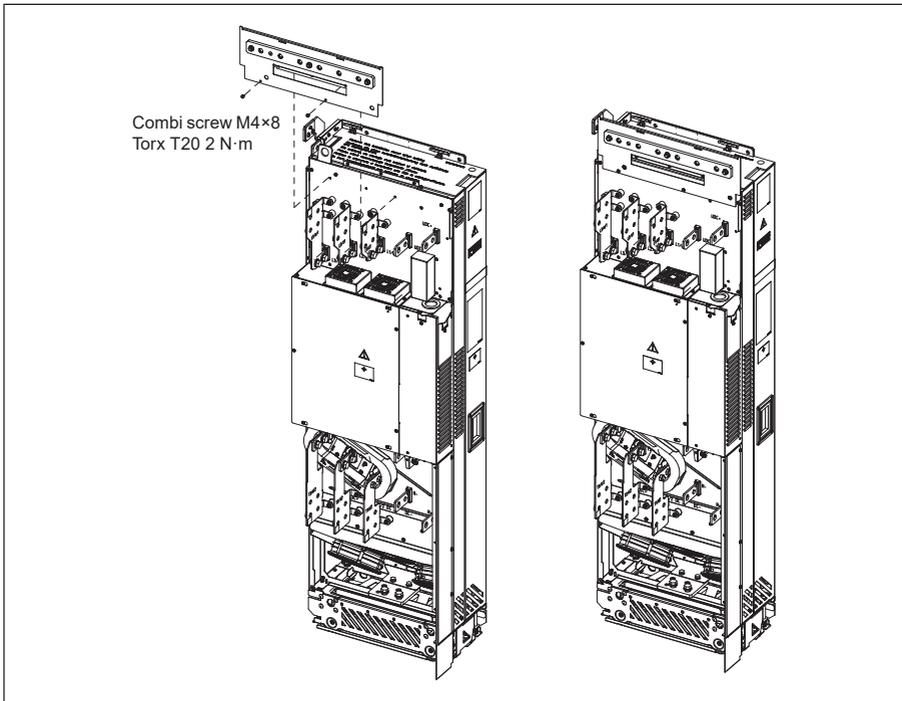
■ **Drive module with full cabling panels (option +H381)**
