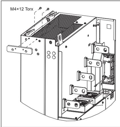
■ **Attaching the drive module to a mounting plate or wall (option +H391)**
