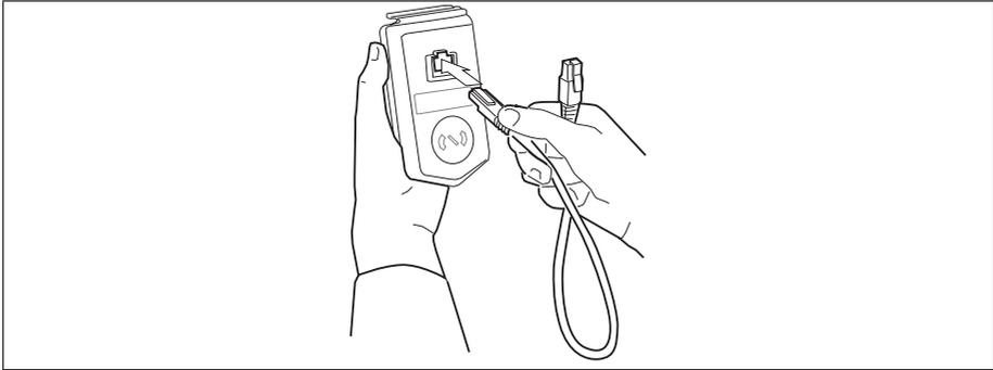
**Note:** When a PC is connected to the control panel, the control panel keypad is disabled. In this case, the control panel acts as a USB-RS485 adapter.
