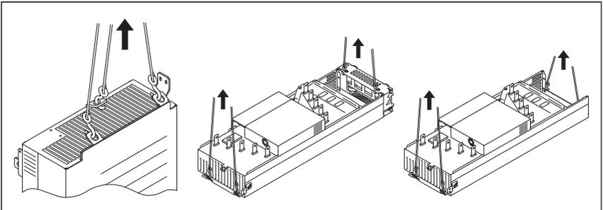
Make sure that the module does not topple over when you move it on the floor: To open the support legs, press each leg a little down (1, 2) and turn it aside. Whenever possible attach the module also with chains. Do not tilt the module. It is heavy and its center of gravity is high. The module overturns from a sideways tilt of 5 degrees. Do not leave the module unattended on a sloping floor.
