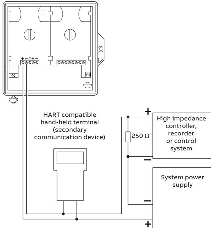
**Figure 2** Analog mode wiring diagram
