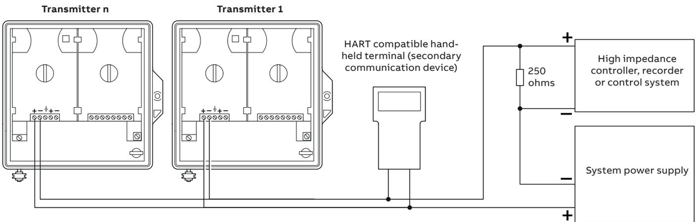
Figure 3 Digital mode wiring diagram
