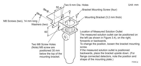
Figure 3.4 Hole Drilling for Plate Mounting
