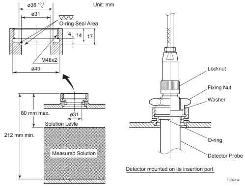
Figure 3.2 Structure of Screw-in Type Detector Mounting Section
