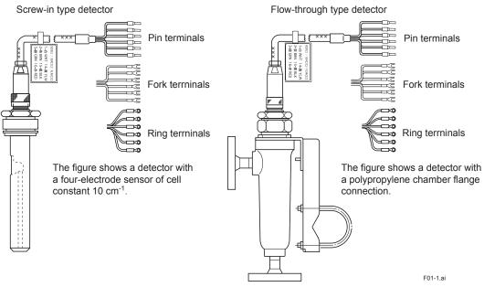
Figure 1.1 External Views of SC8SG Conductivity Detectors (example)
