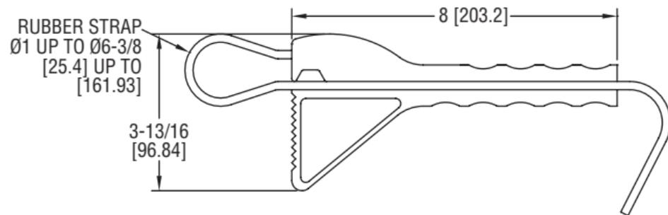
The **MODEL SWUK1** offers the user a versatile tool to grip, undo & tighten a wide variety of awkwardly shaped and sized objects. The SWUK1 also makes the job of fitting Adjustable Signal Flags (ASF) covers to Magnehelic® Differential Pressure Gages much easier by simply following the instruction included with each cover supplied.
