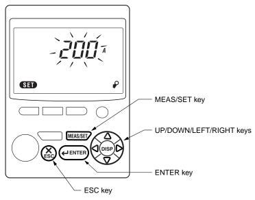
(2) Using the △ ▽ < ○ keys, select the number corresponding to the desired clamp-on current probe. The number changes sequentially as follows.</p>
