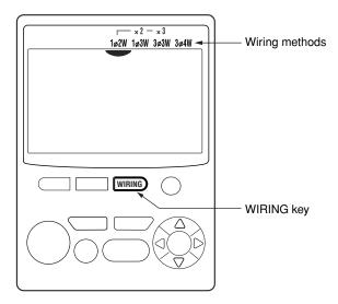
To change the wiring method, press the **V**Range key. Each time you press the WIRING key, the — moves to change the selected wiring method.
