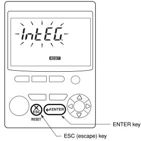
(2) Press the eleverst key. The electric energy count is cleared and the measurement screen returns. To cancel, press the key. The measurement screen also returns.
