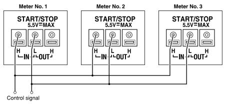
• Controlling Meter Nos. 2 and 3 by Control Signal of Meter No. 1
