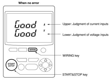
When an error is displayed, refer to the table on page 5-8 and check the meaning of the error. Check and correct the connections, then press the (START) key to carry out the wiring check again.
