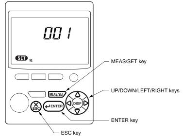
(2) Using the  $\triangle \bigtriangledown \lhd \bigcirc$  keys, select the desired item, and then press the events key. Each time one of the  $\triangle \bigtriangledown \lhd \bigcirc$  keys is pressed, the setting item changes sequentially as follows.
