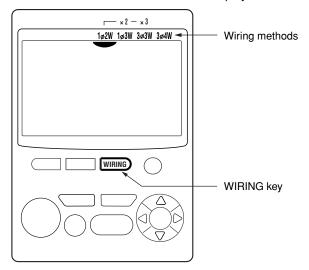
Each press of the WIRING key changes the wiring method selection sequentially as follows:
