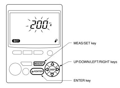
(3) Using the  $\triangle \bigtriangledown \lhd \bigcirc$  keys, select the number corresponding to the desired clamp-on current probe.
