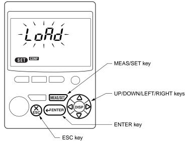
(2) Using the  $\bigcirc$  keys, select  $L \Box A d$  or  $S A \sqcup E$ .
