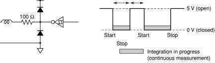
Remote integration start/stop control takes precedence over manual start/ stop and automatic start/stop at specified times. Remote control takes effect even during the integration standby state and when a setting screen is displayed. However, it is ineffective when integration has already begun and is on.
