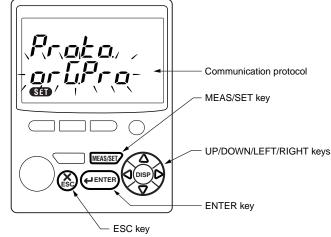
(2) Using the  $\triangle \bigtriangledown \lhd \circlearrowright$  keys, select the communication protocol. The displayed communication protocol changes sequentially as follows.
