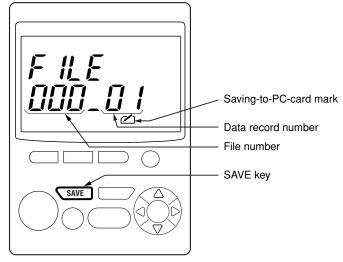
(2) Pressing the SAVE key again saves the measured values again with the data record number incremented but with the file number unchanged.
