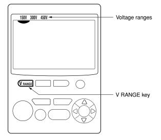
Each press of the  $\overline{v_{\text{Range}}}$  key changes the range selection sequentially as follows:
