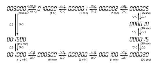
(3) After selecting the desired interval, press the *entry* key. The interval is changed accordingly and the setting item selection screen returns. To cancel the change, press the *k* key. The setting item selection screen also returns.
