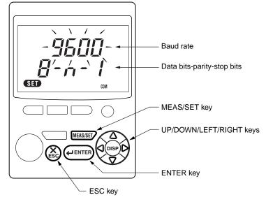
(2) If necessary, change the baud rate using the  $\triangle \bigtriangledown$  keys. The baud rate changes sequentially as follows.
