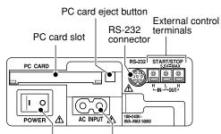
Power switch Power supply connector Model with RS-232 interface
