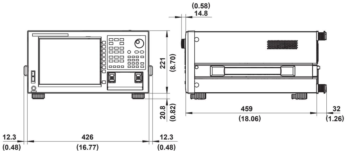
If not specified, the tolerance is  $\pm 3\%$ . However, in cases of less than 10 mm, the tolerance is  $\pm 0.3$  mm.
