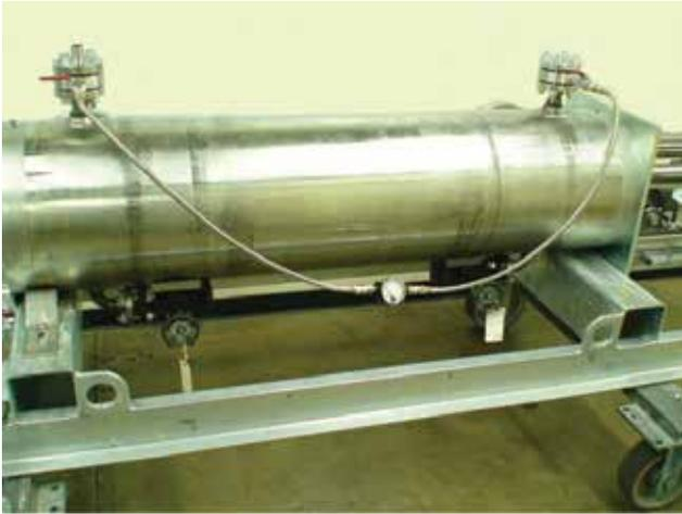
Figure 5-1: Static Leak Detection Set-up
