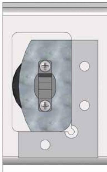
Figure 8-30: Correct Optical Switch Installation Bottom View
