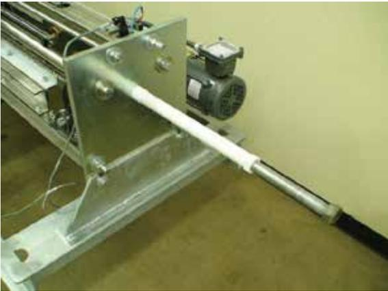
Figure 5-3: Differential pressure creator inserted in drive end plate.
