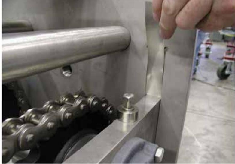
**Figure 8-21:** Inserting Shim behind Side Plate
