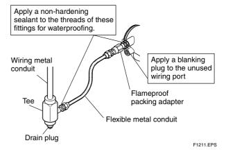
Figure 12.4.2 Typical Wiring Using Flexible Metal Conduit
