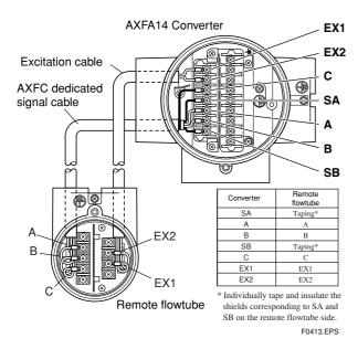
Figure 4.4.5 Wiring Diagram
