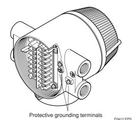
Figure 4.4.4 Protective Grounding Terminal Location
