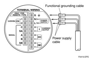
Figure 4.4.3 Electric Cable Wiring
