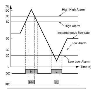
Select "H/L Alarm(O)" for **F20: DO Function** Select "HH/LL Alarm(O)" for **F21: DIO Function** Select "Closed (On) Act" for **F22: DO Active Mode** Select "Closed/Short Act" for **F23: DIO Active Mode**
