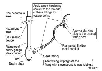
Figure 12.4.4 Typical Wiring Using Flameproof Metal Conduit
