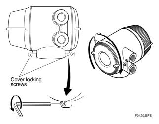
Figure 4.4.12 Installing the Terminal Box Cover
