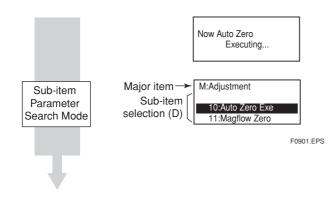
Auto zero adjustment function is being executed (about 30 seconds).
