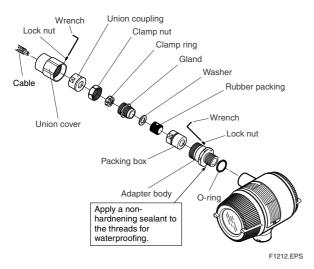
Figure 12.4.3 Installing Flameproof Packing Adapter
