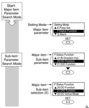
Once in Setting Mode, use the switch to move the cursor to **F: Status Function**.
