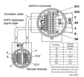
Figure 4.4.6 Wiring Diagram
