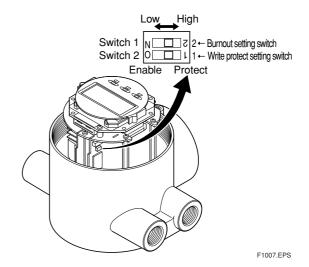
Figure 10.2.1 Switch Configuration
