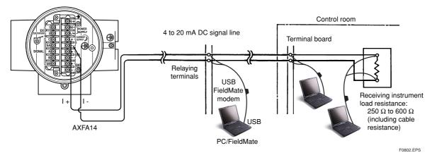
Figure 8.2.1 Interconnection Diagram
