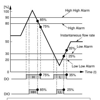
Select "H/L Alarm(O)" for F20: DO Function Select "HH/LL Alarm(O)" for F21: DIO Function Select "Closed (On) Act" for F22: DO Active Mode Select "Closed/Short Act" for F23: DIO Active Mode
