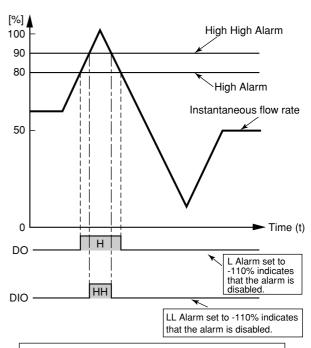
Select "H/L Alarm(O)" for F20: DO Function Select "HH/LL Alarm(O)" for F21: DIO Function Select "Closed (On) Act" for F22: DO Active Mode Select "Closed/Short Act" for F23: DIO Active Mode
