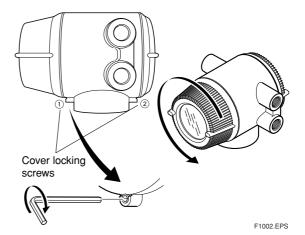
Figure 10.1.1 Removing the Display Cover
