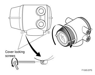
Figure 10.1.3 Installing the Display Cover
