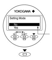
A screen is displayed to confirm whether or not the system is to enter Setting Mode.
