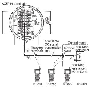
Figure 7.2 Connecting the BT200
