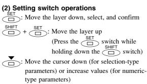
SHIFT : Move the cursor to the right (for numeric-type parameters)
