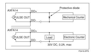
Figure 4.4.8 Pulse Output Connection
