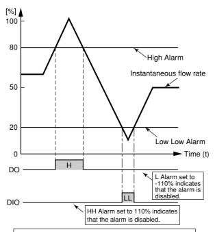
Select "H/L Alarm(O)" for **F20: DO Function** Select "HH/LL Alarm(O)" for **F21: DIO Function** Select "Closed (On) Act" for **F22: DO Active Mode** Select "Closed/Short Act" for **F23: DIO Active Mode**
