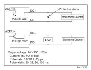
Figure 4.4.9 Active Pulse Output Connection (Optional code EM)
