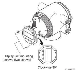
Figure 10.1.2 Changing the Display Unit Direction 90 Degrees
