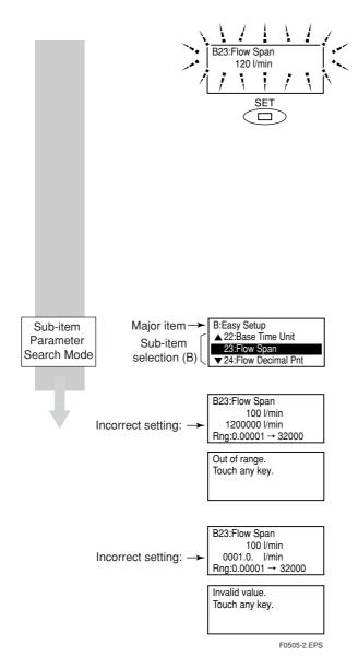
When the switch is touched, the entire display flashes on and off. Confirm that the setting has been correctly changed to "120", and then fix this value by touching the switch once again.
