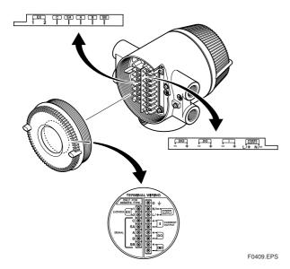
Figure 4.4.2 Terminal Layout Labels Position
