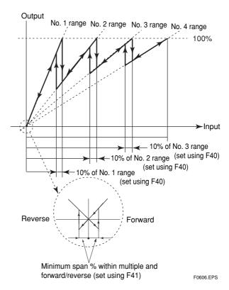
Figure 6.4.1 Multiple Ranges and Hysteresis Widths
