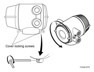
Figure 4.4.1 Removing the Terminal Box Cover
