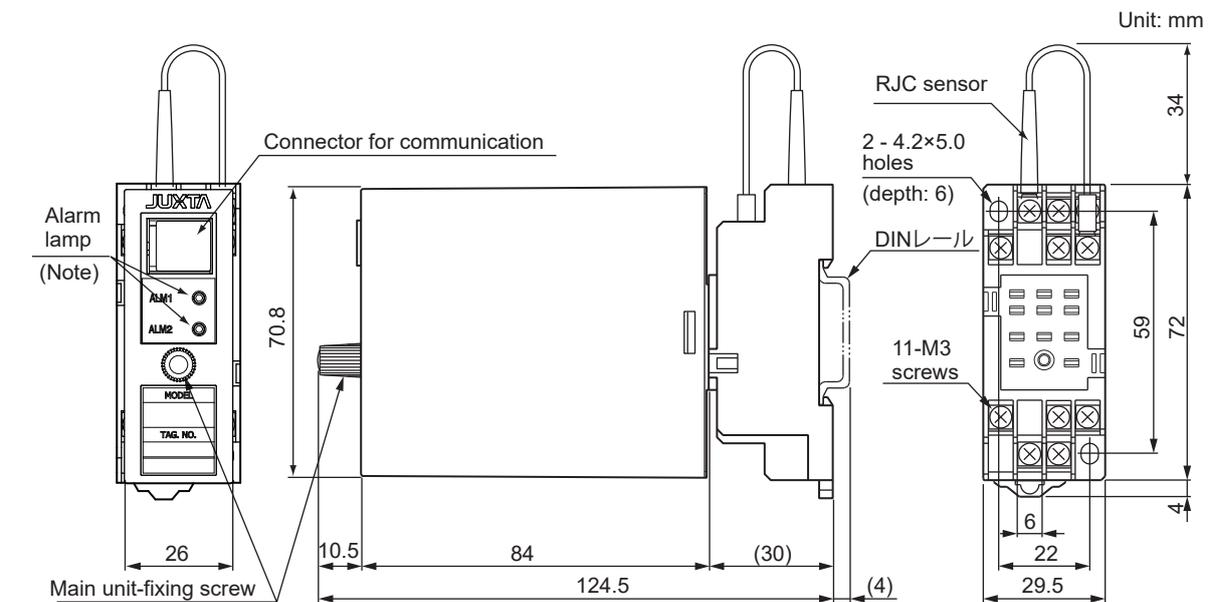
Note: Only when output-2 is alarm output
